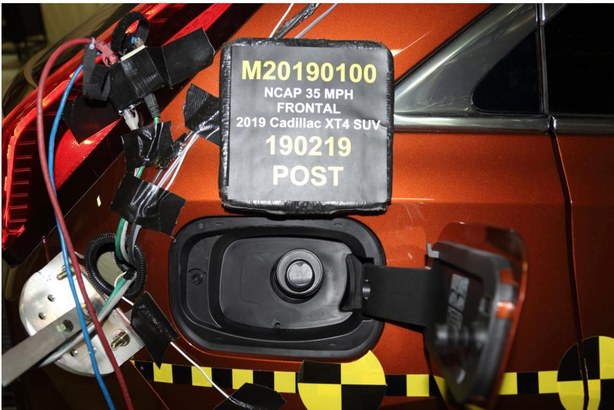
**023 Post-Test Fuel Filler Cap View**
