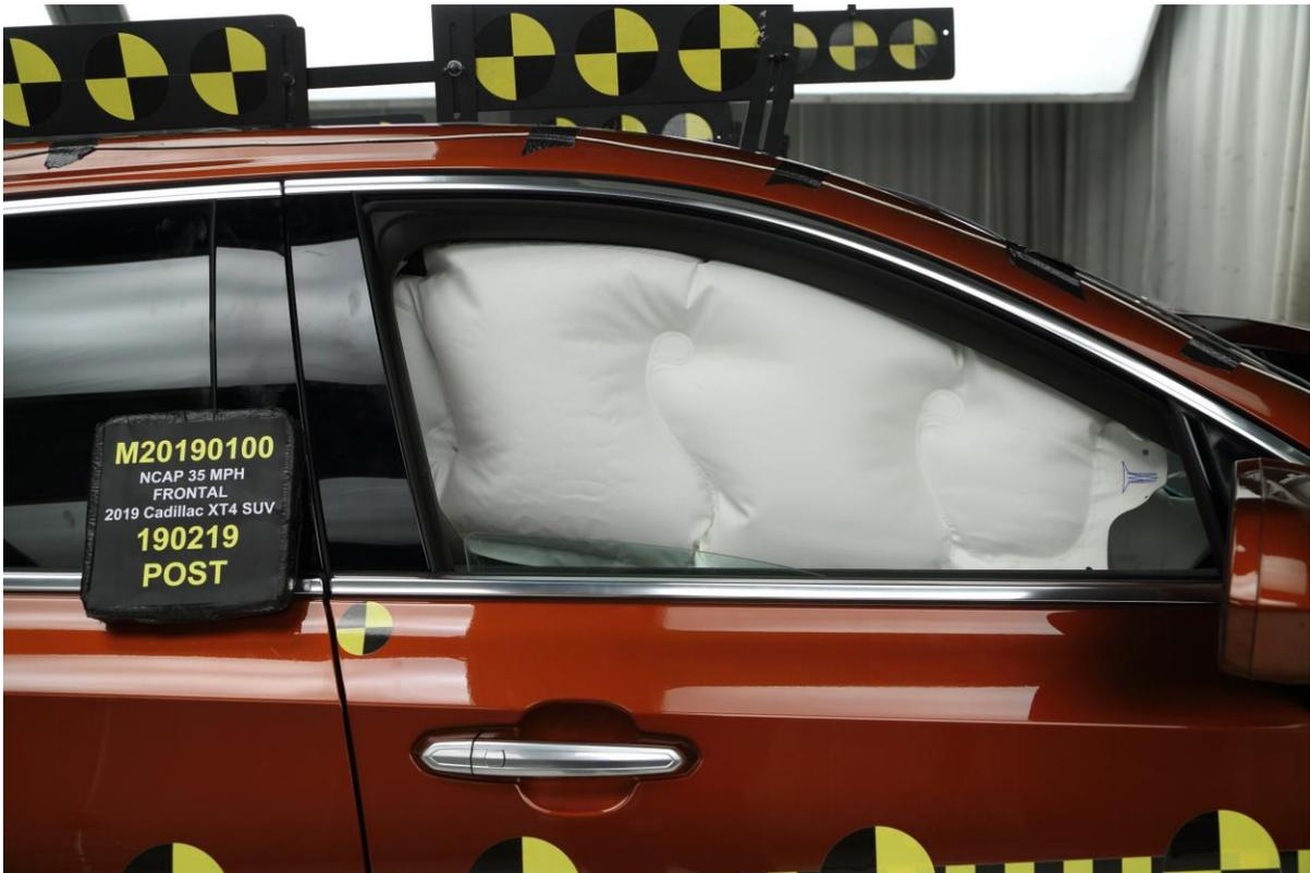
**056 Post-Test Passenger Dummy Window View**
