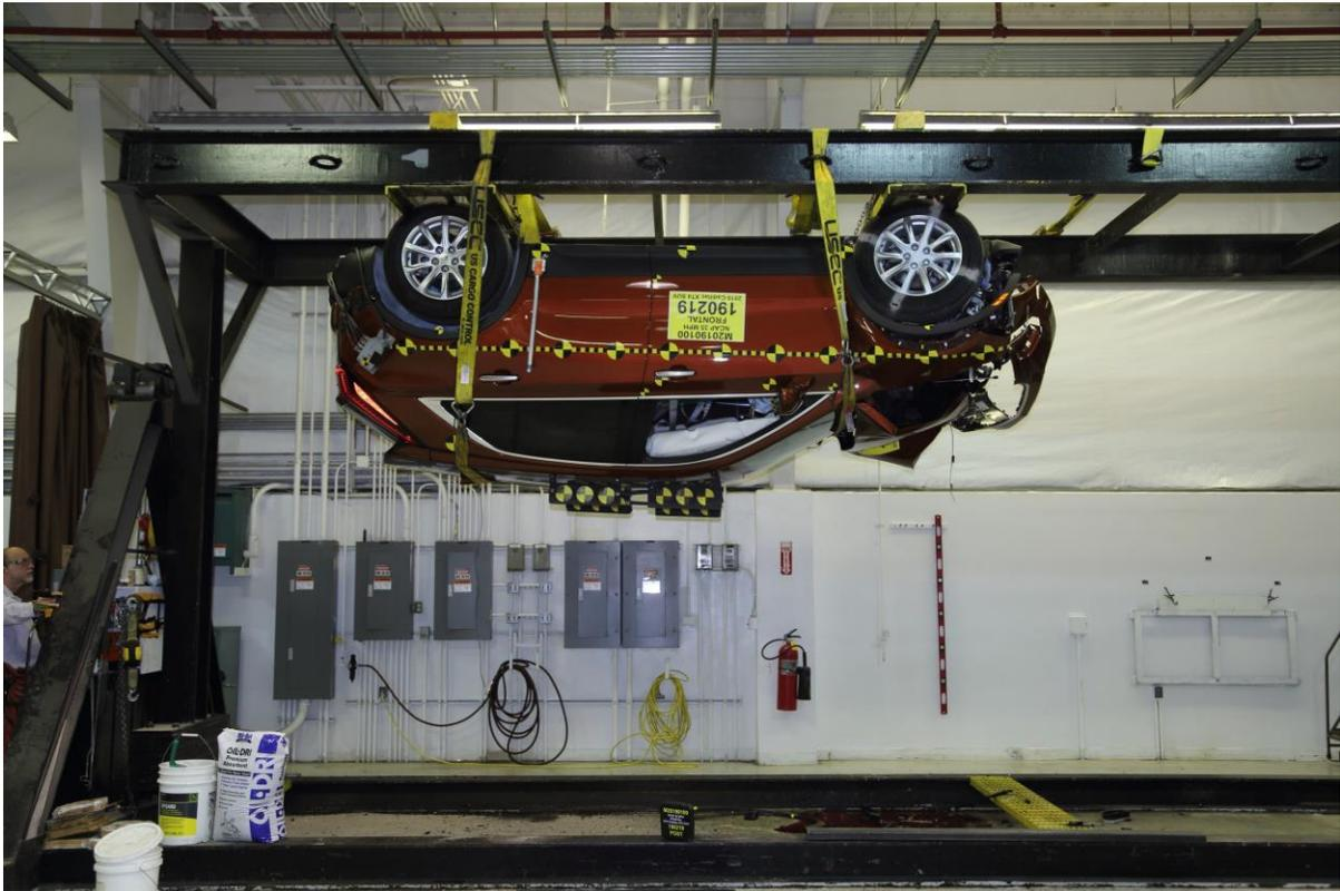
**079 Vehicle at 180° on Static Rollover Device**
