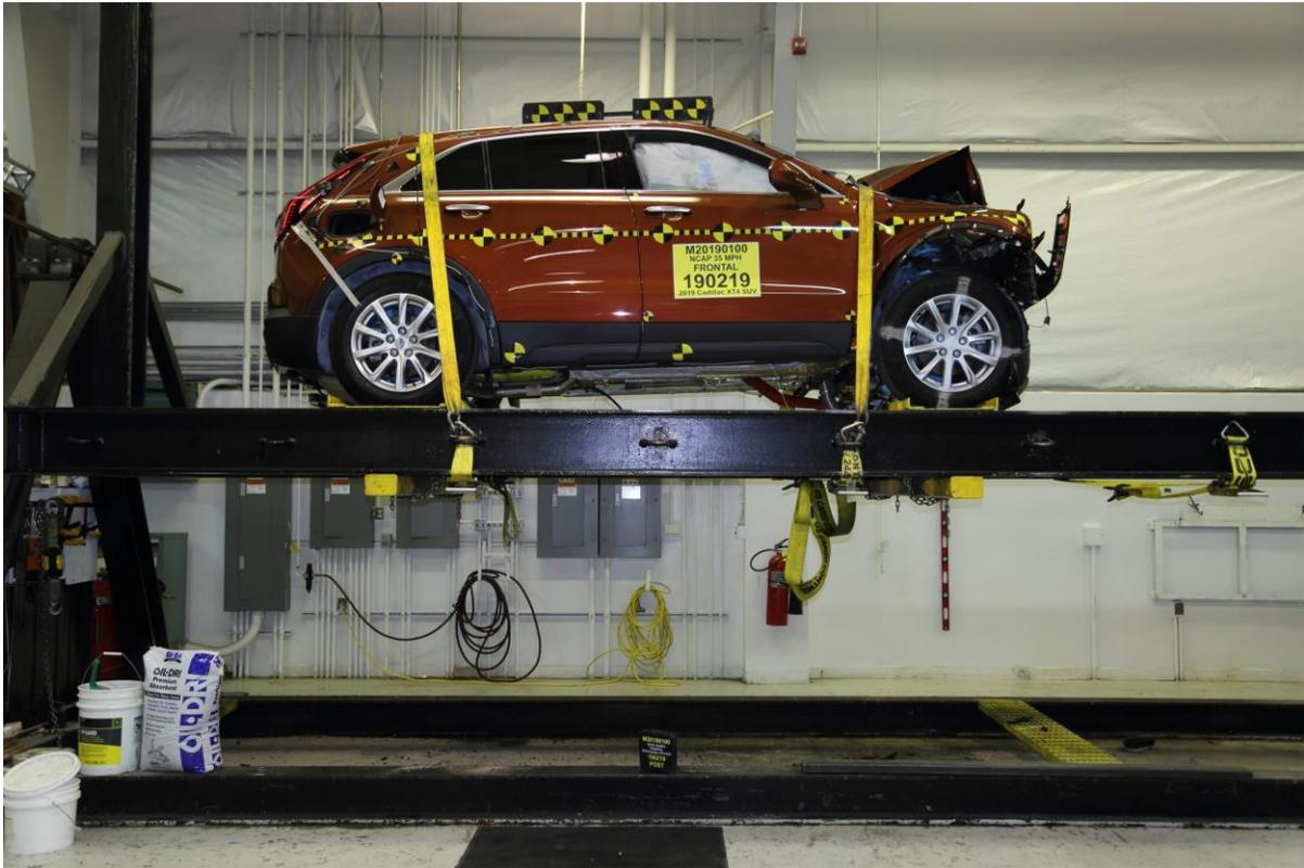
**077 Vehicle at 0° on Static Rollover Device**
