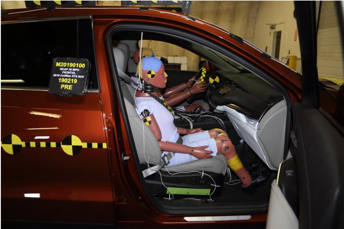
**057 Pre-Test Passenger Dummy and Vehicle Interior View**
