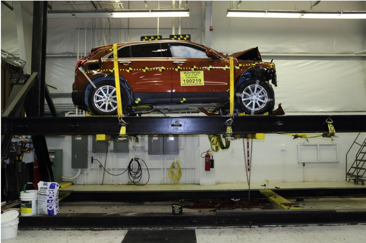
**081 Vehicle at 360° on Static Rollover Device**
