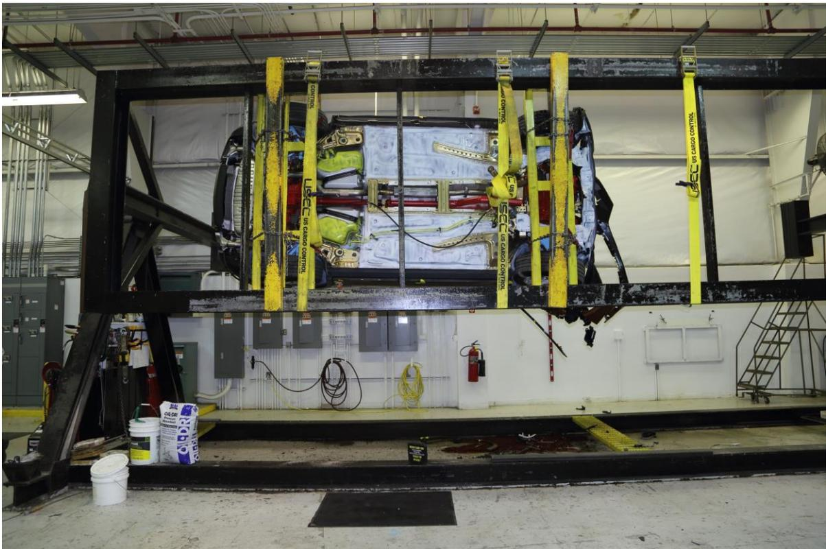
**080 Vehicle at 270° on Static Rollover Device**
