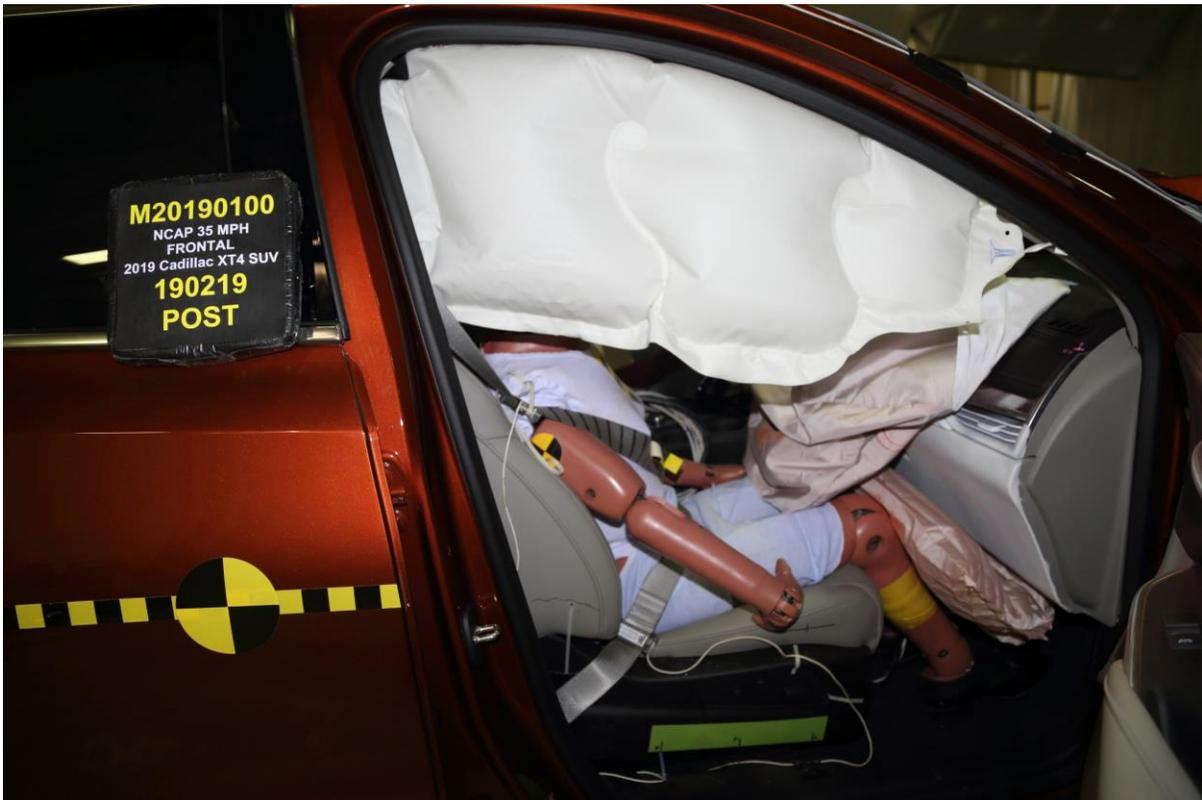
**058 Post-Test Passenger Dummy and Vehicle Interior View**
