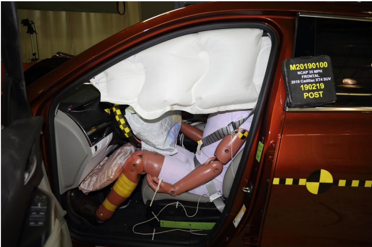
**035 Post-Test Driver Dummy and Vehicle Interior View**
