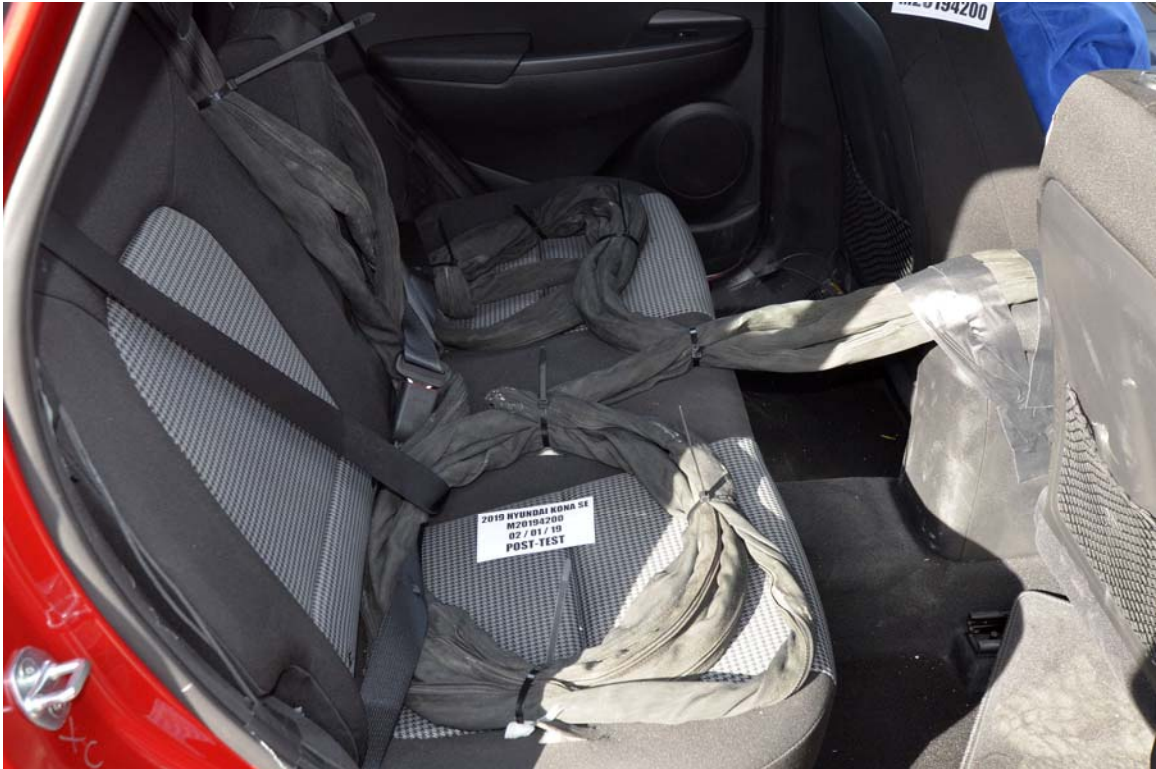
FIGURE 29. Post-Test Dummy Cable Routing
