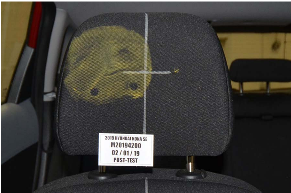
FIGURE 48. Post-Test Driver Dummy Contact with Headrest
