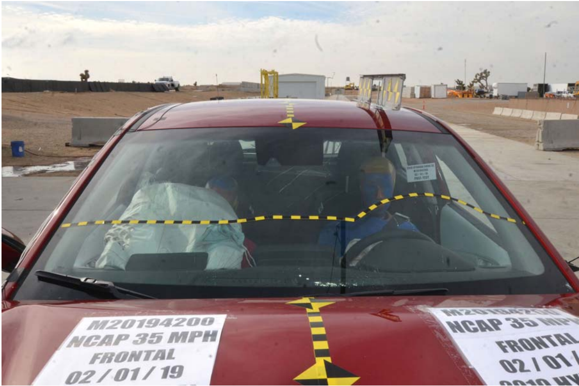
FIGURE 19. Post-Test Windshield View
