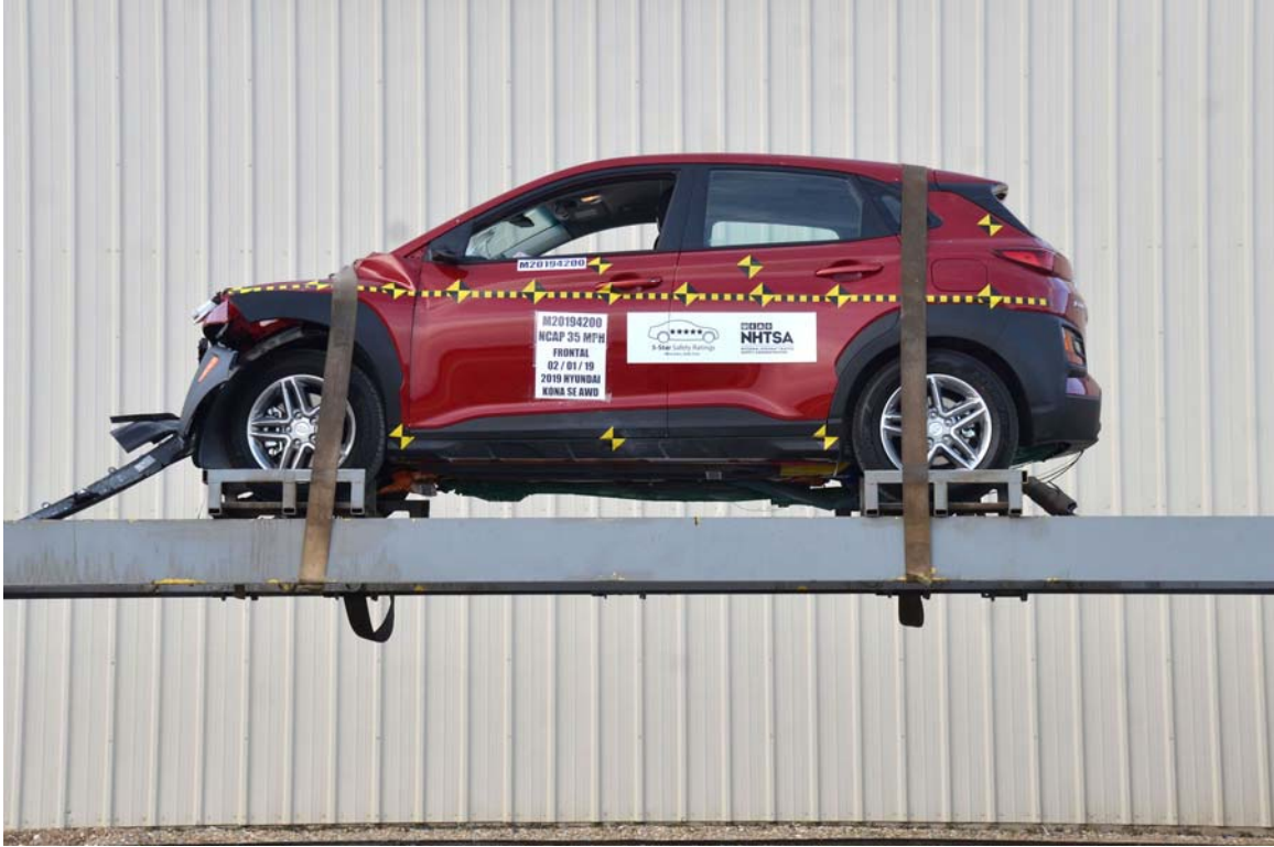
FIGURE 73. Vehicle at 0° on Static Rollover Device
