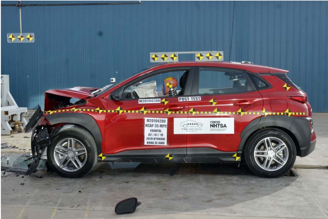
FIGURE 11. Post-Test Left View of Test Vehicle
