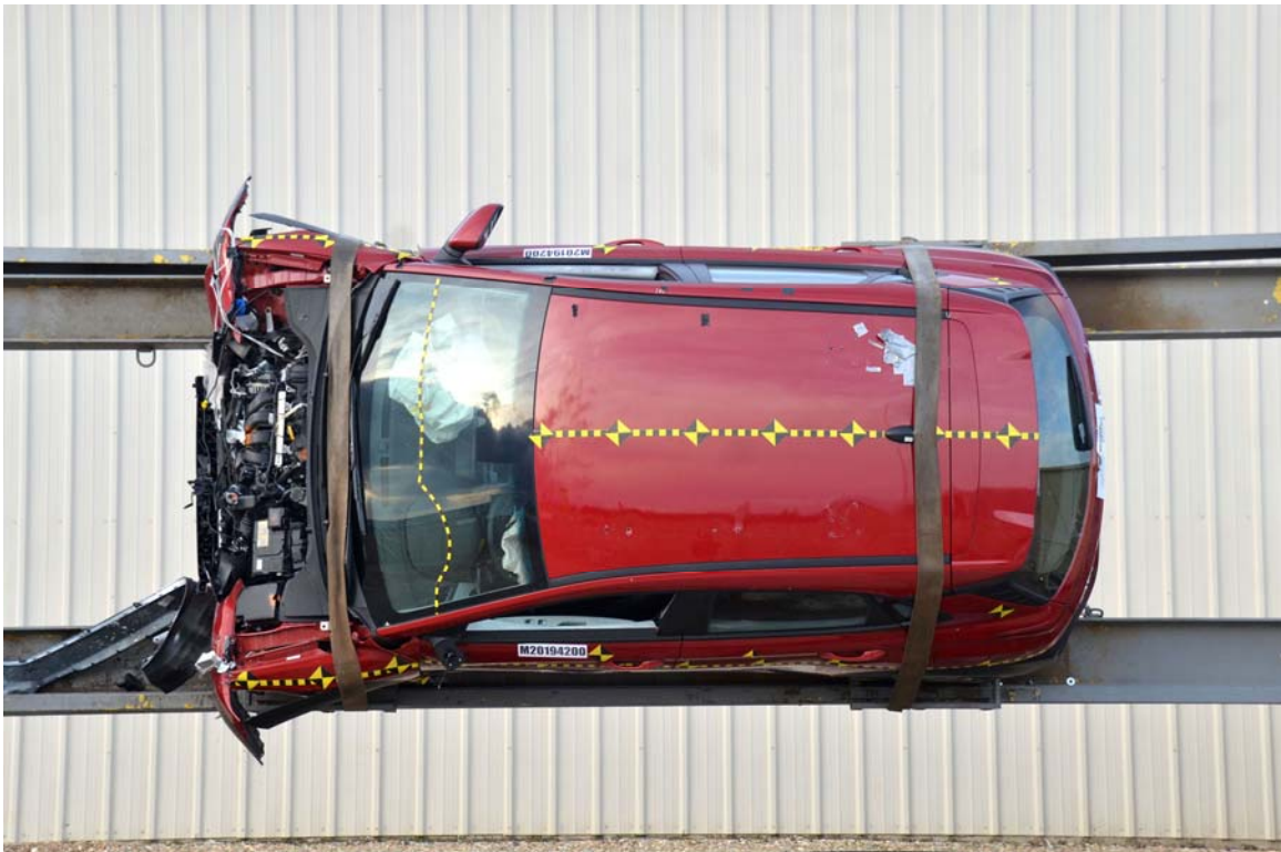
FIGURE 74. Vehicle at 90° on Static Rollover Device
