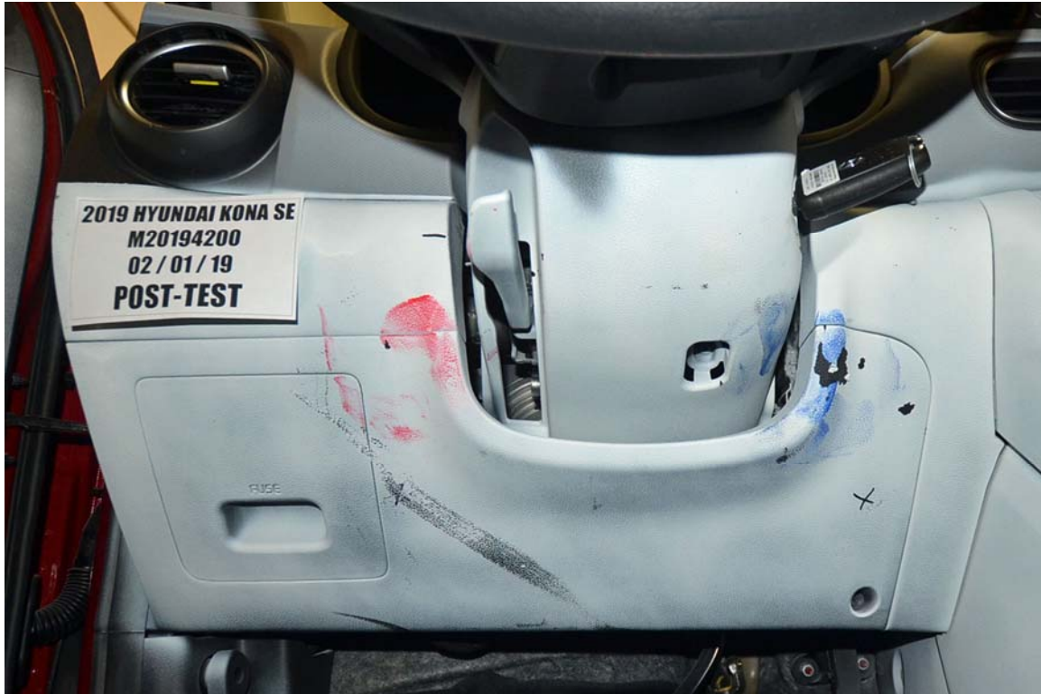
FIGURE 43. Post-Test Driver's Side Knee Bolster
