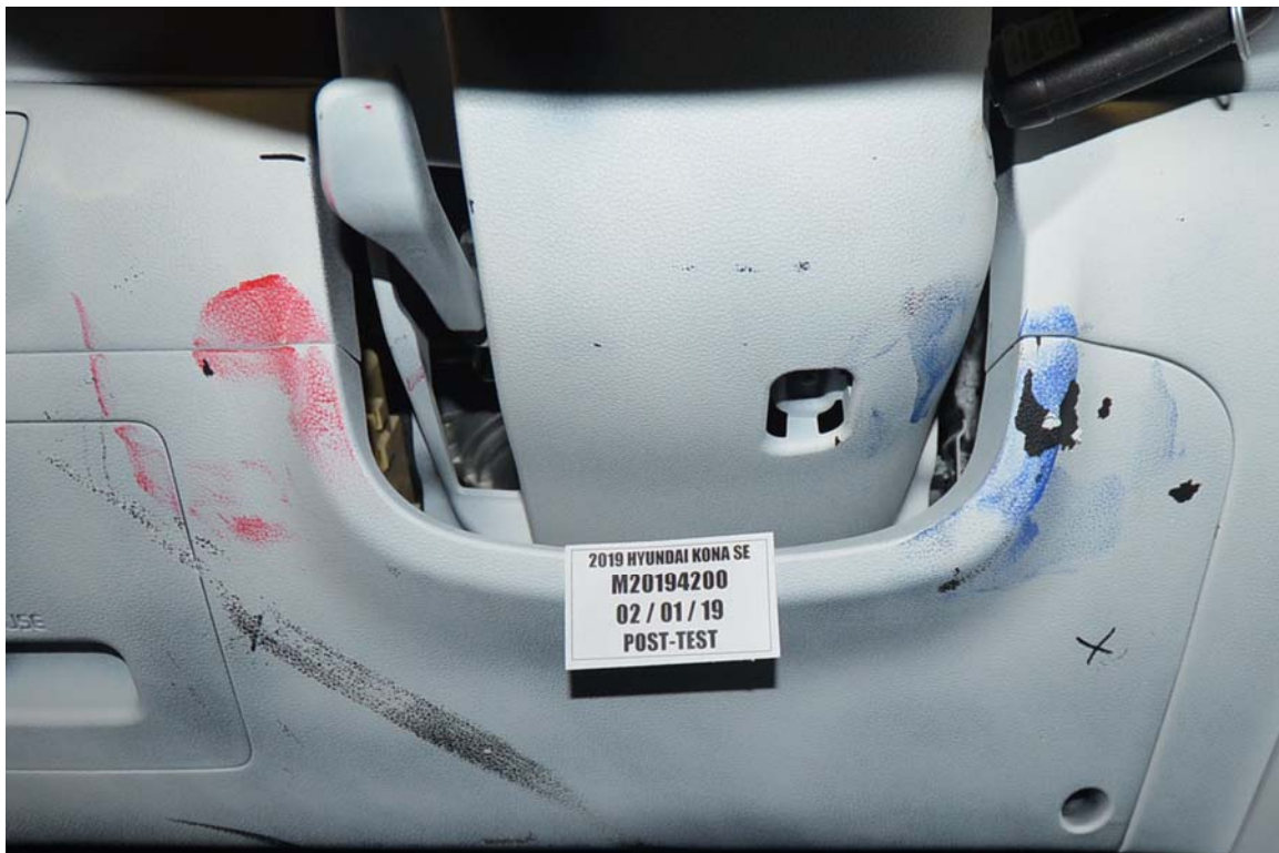
FIGURE 48b. Post-Test Driver Dummy Contact with Knee Bolster
