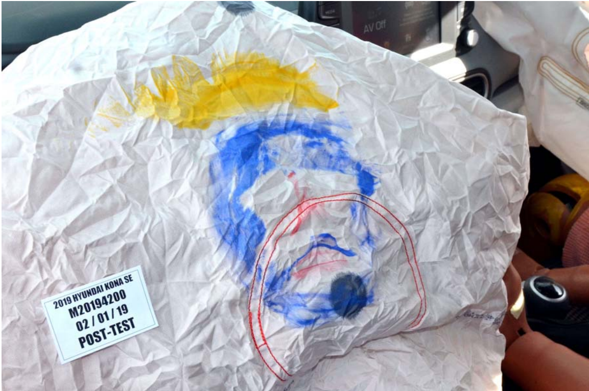
FIGURE 47. Post-Test Driver Dummy Contact with Airbag
