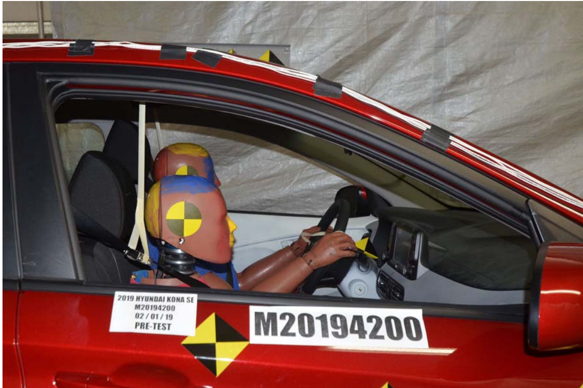
FIGURE 53. Pre-Test Passenger Dummy Window View
