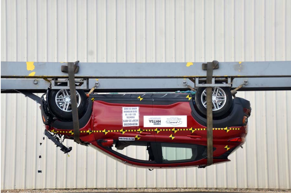
FIGURE 75. Vehicle at 180° on Static Rollover Device
