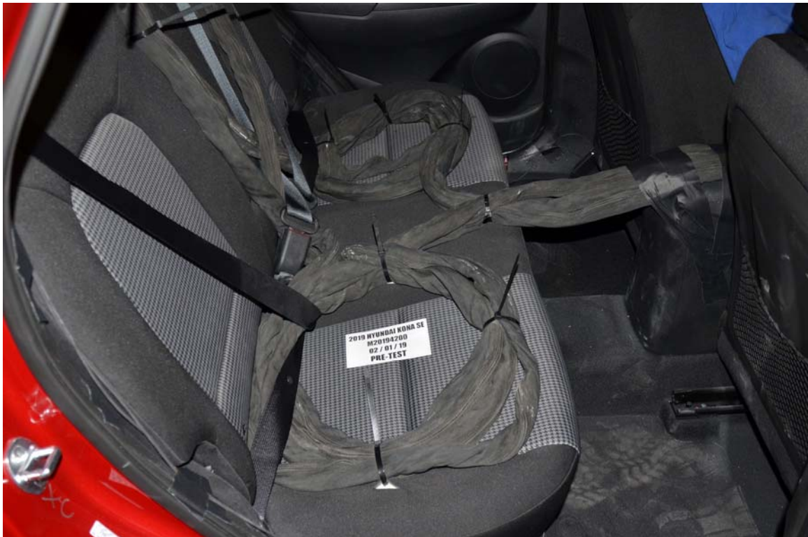
FIGURE 28. Pre-Test Dummy Cable Routing
