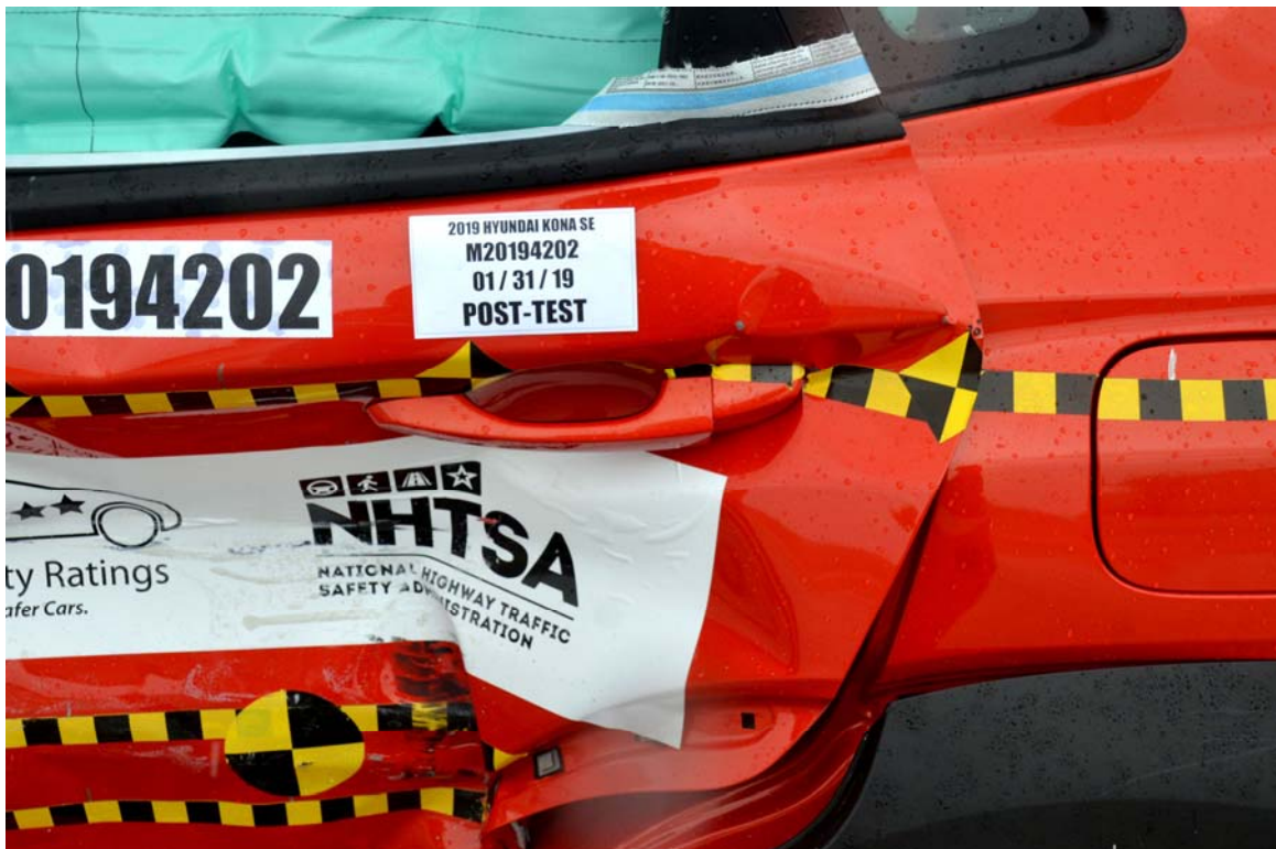
FIGURE 24. Post-Test Left Rear Door Latch Close-Up
