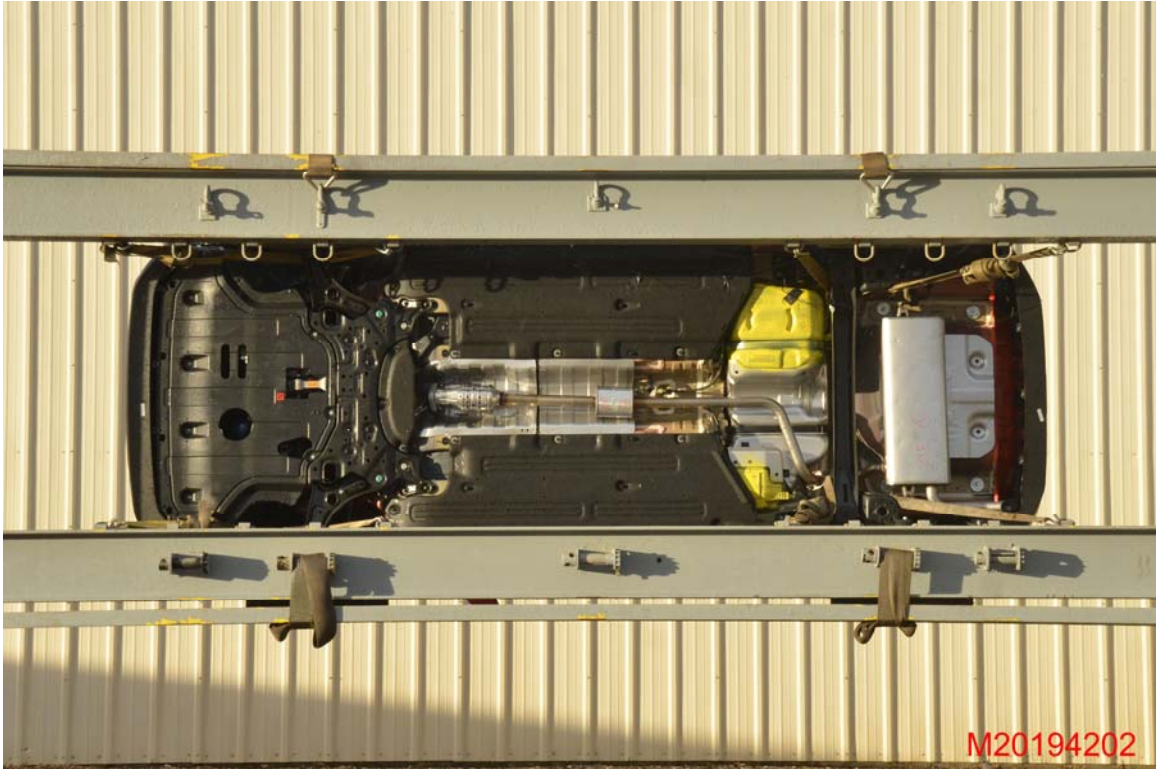
FIGURE 99. FMVSS No. 301 Static Rollover 270 Degrees
