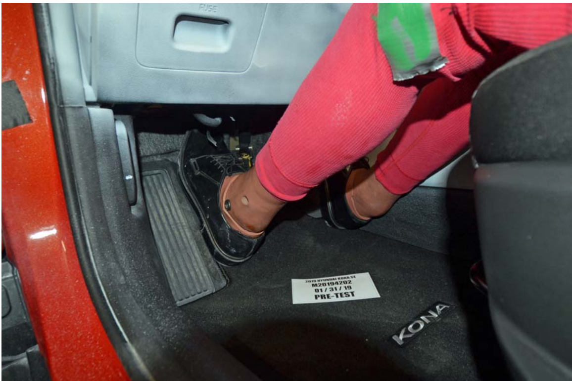
FIGURE 34. Pre-Test Placement of Driver Dummy's Feet
