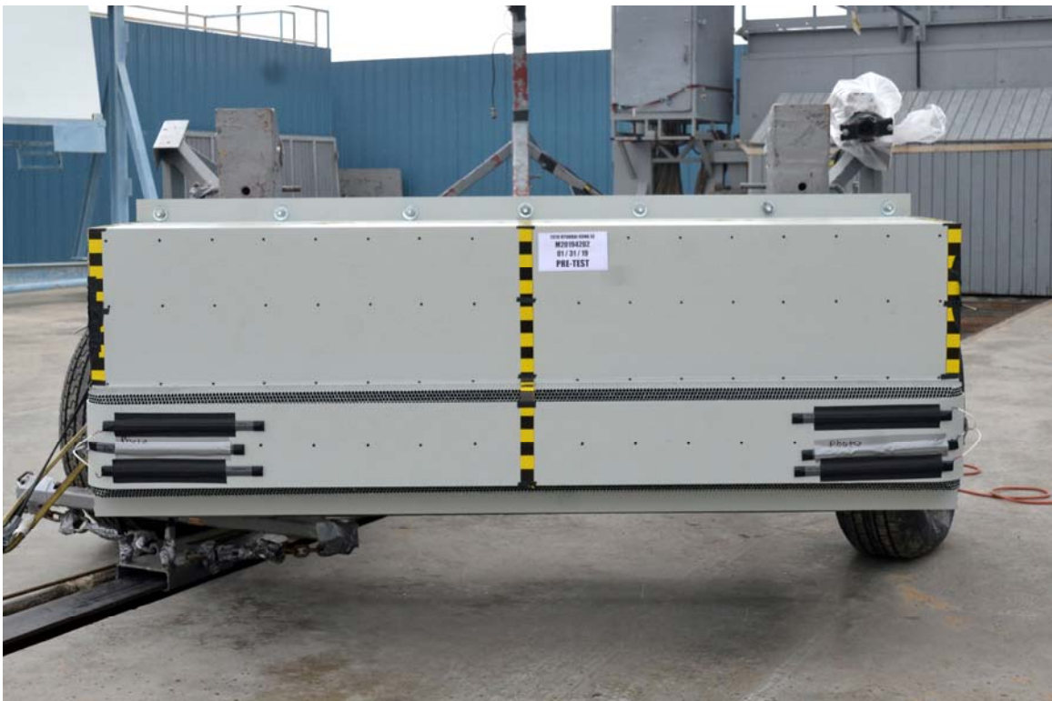
FIGURE 84. Pre-Test Front View of MDB Impactor Face
