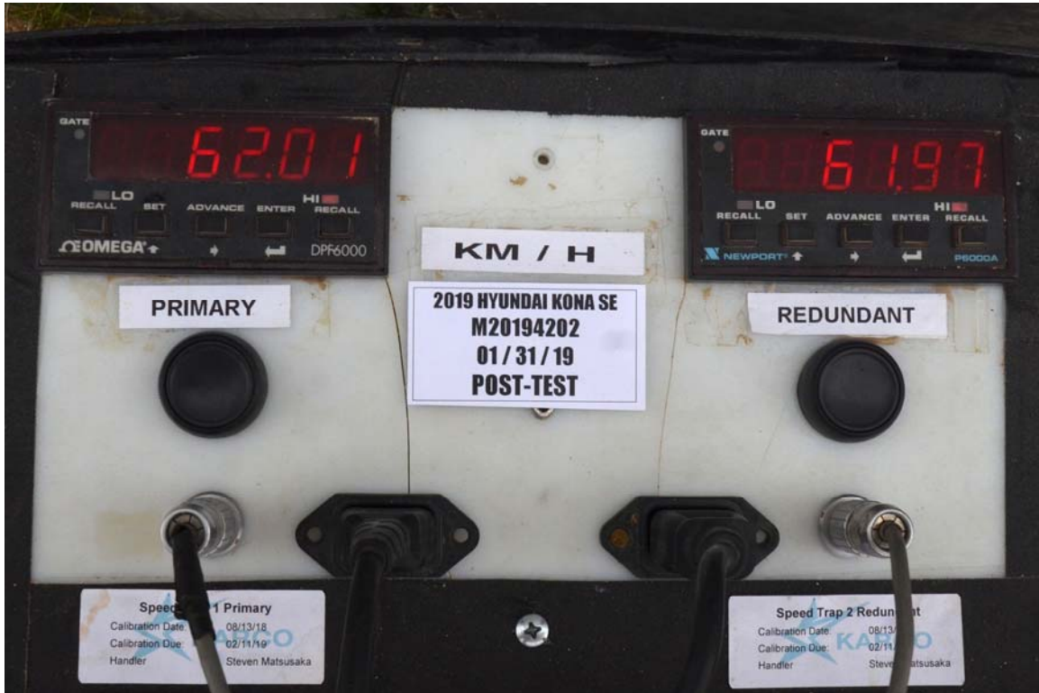
FIGURE 95. Post-Test Primary and Redundant Speed Trap Read-Out
