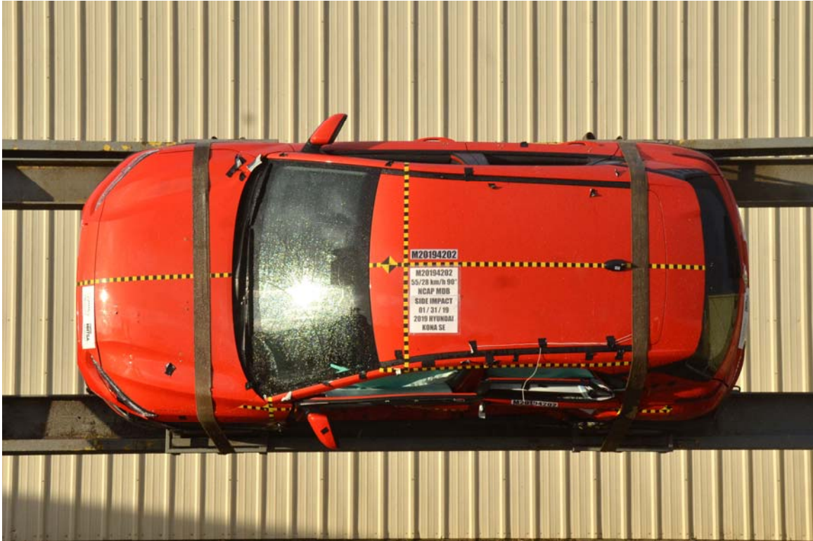
FIGURE 97. FMVSS No. 301 Static Rollover 90 Degrees
