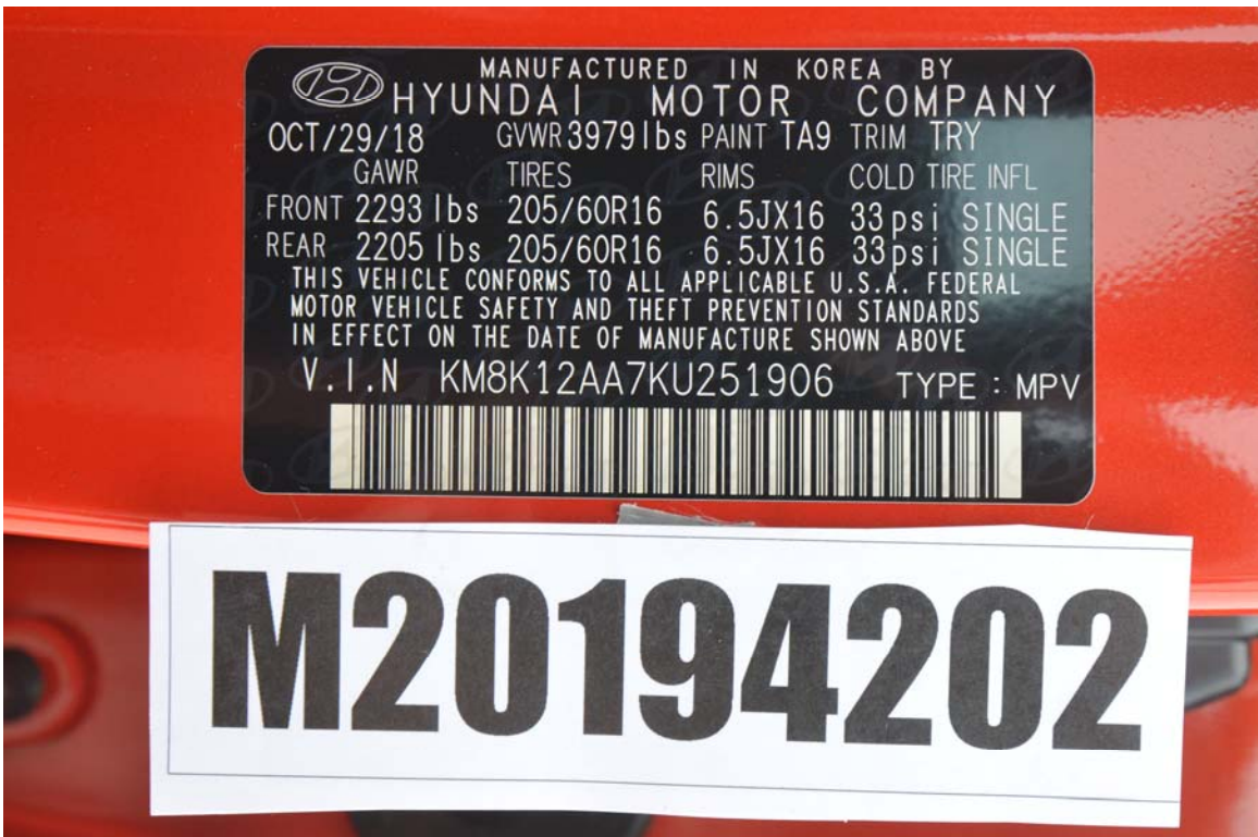
FIGURE 92. Close-Up View of Vehicle's Certification Label
