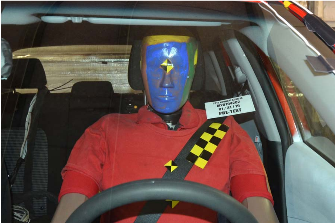
FIGURE 25. Pre-Test Front Close-Up View of Driver Dummy
