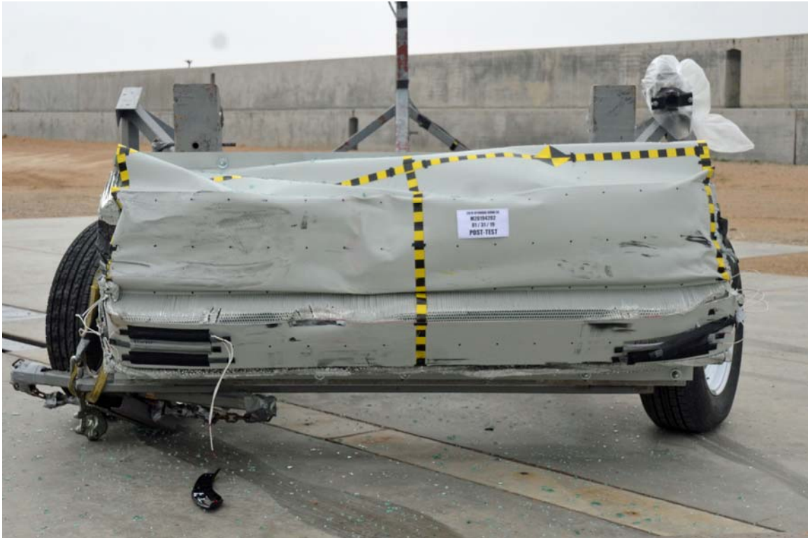
FIGURE 85. Post-Test Front View of MDB Impactor Face
