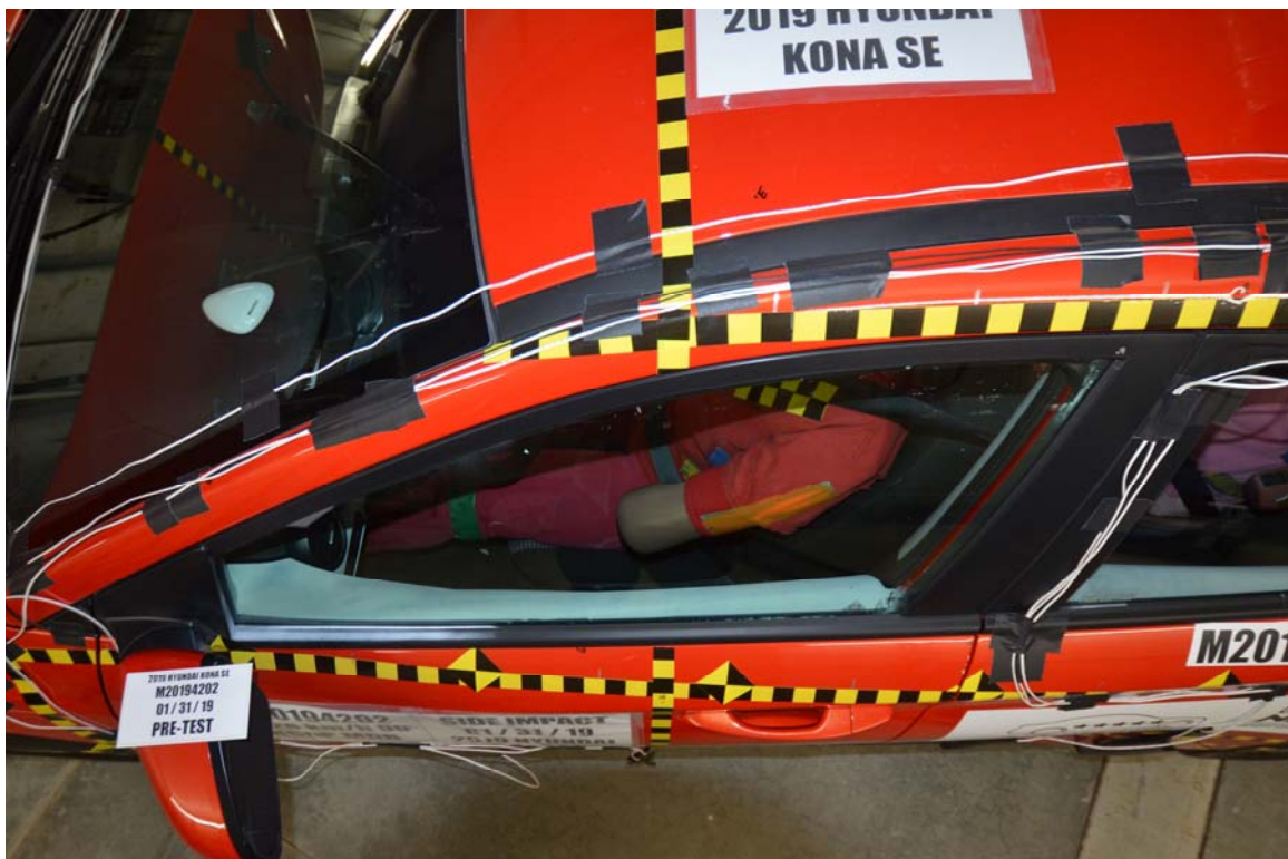
FIGURE 42. Pre-Test Driver Dummy and Door Clearance View
