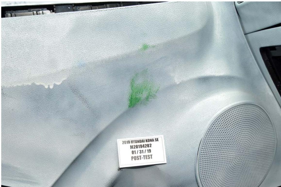
FIGURE 54. Post-Test Driver Dummy Close-Up Knee Contact View
