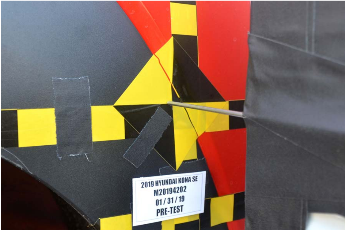
FIGURE 19. Pre-Test Close-Up View of Impact Point Target
