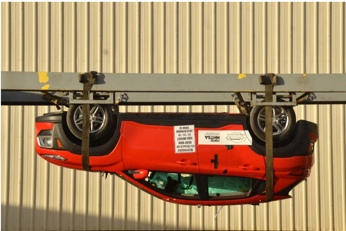
FIGURE 98. FMVSS No. 301 Static Rollover 180 Degrees
