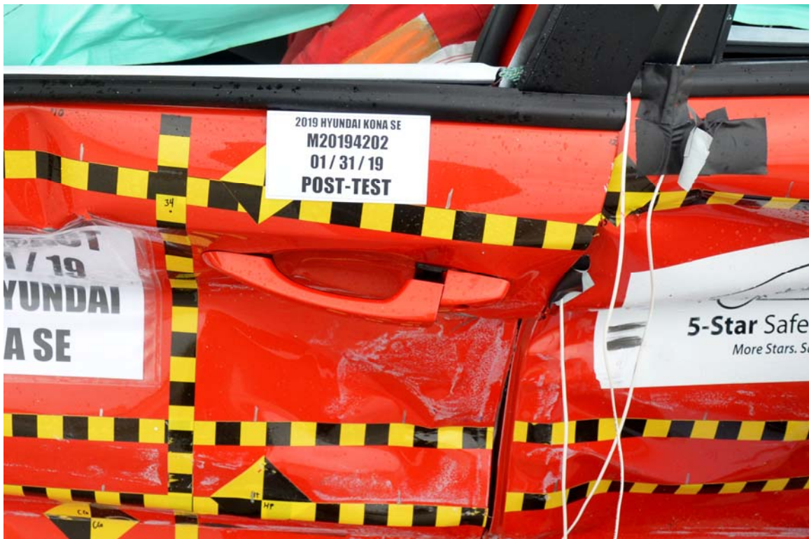
FIGURE 22. Post-Test Left Front Door Latch Close-Up
