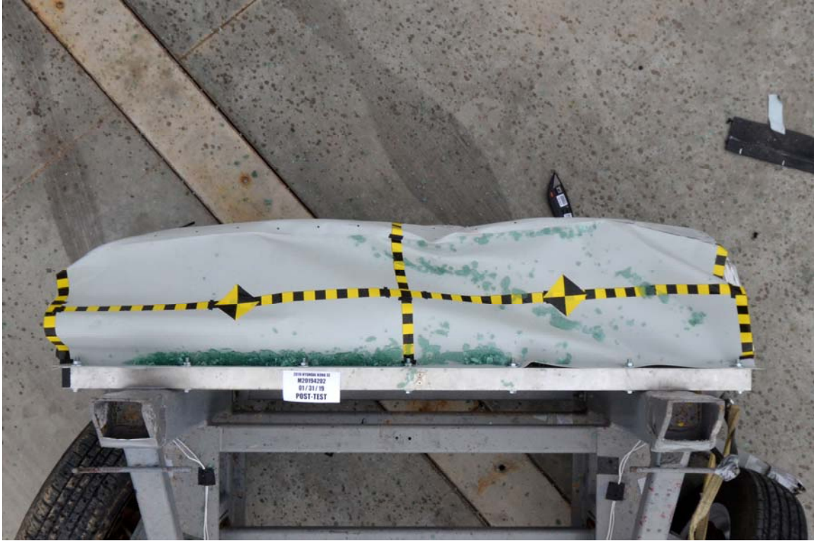
FIGURE 87. Post-Test Top View of MDB Impactor Face
