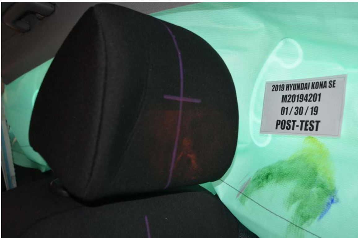
FIGURE 46. Post-Test Dummy Close-Up Head Contact with Vehicle Interior View
