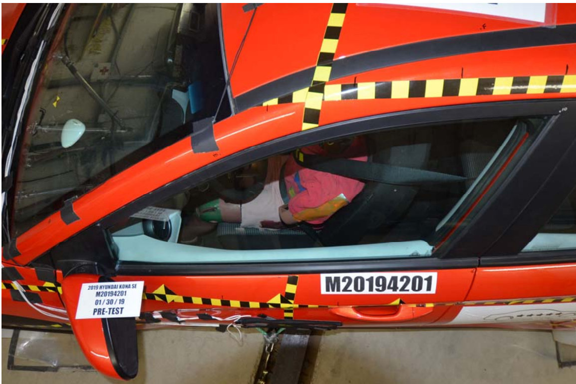
FIGURE 40. Pre-Test Dummy and Door Clearance View
