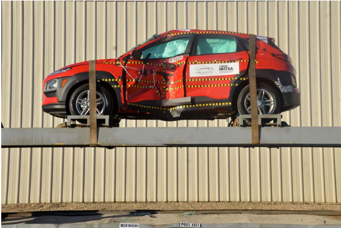
FIGURE 67. FMVSS No. 301 Static Rollover 360 Degrees
