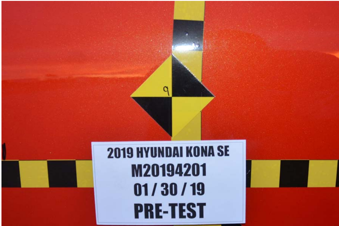
FIGURE 19. Pre-Test Close-Up View of Impact Point Target
