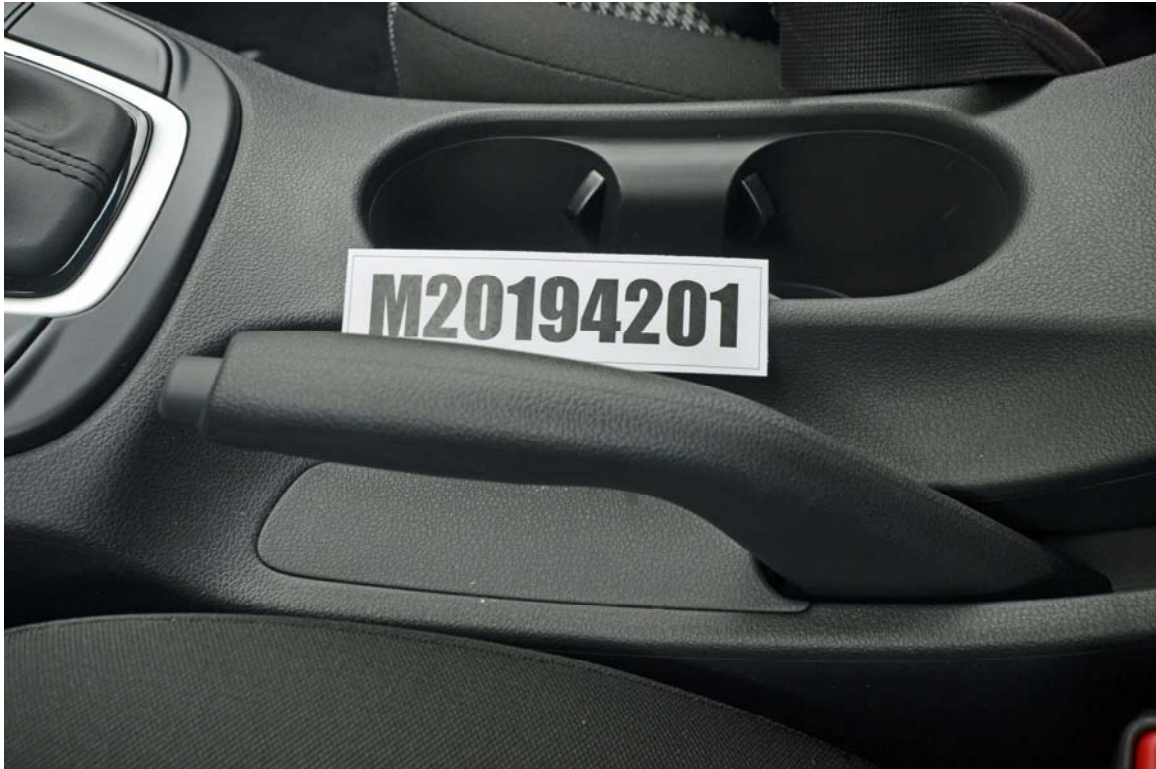
FIGURE 35. View of Disengaged Parking Brake
