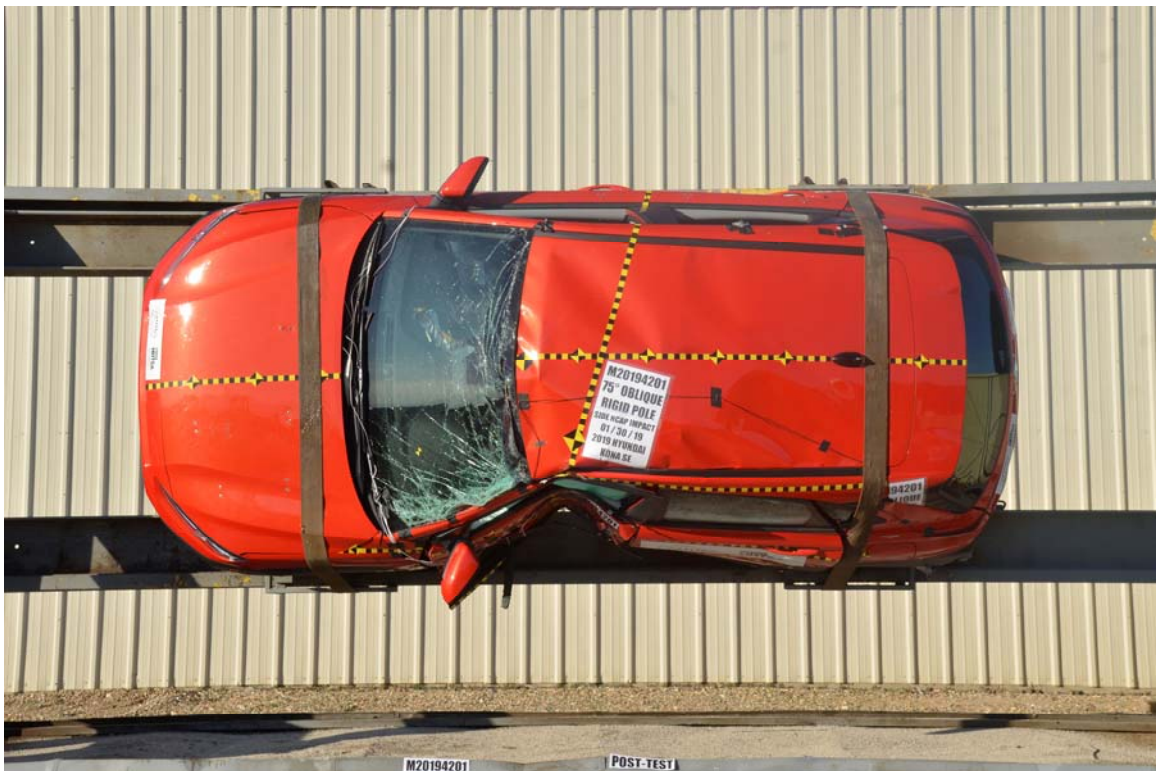
FIGURE 64. FMVSS No. 301 Static Rollover 90 Degrees
