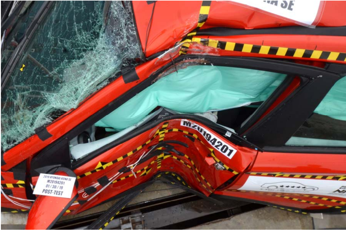
FIGURE 41. Post-Test Dummy and Door Clearance View
