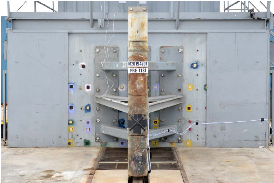
FIGURE 57. Pre-Test Pole Barrier Front View
