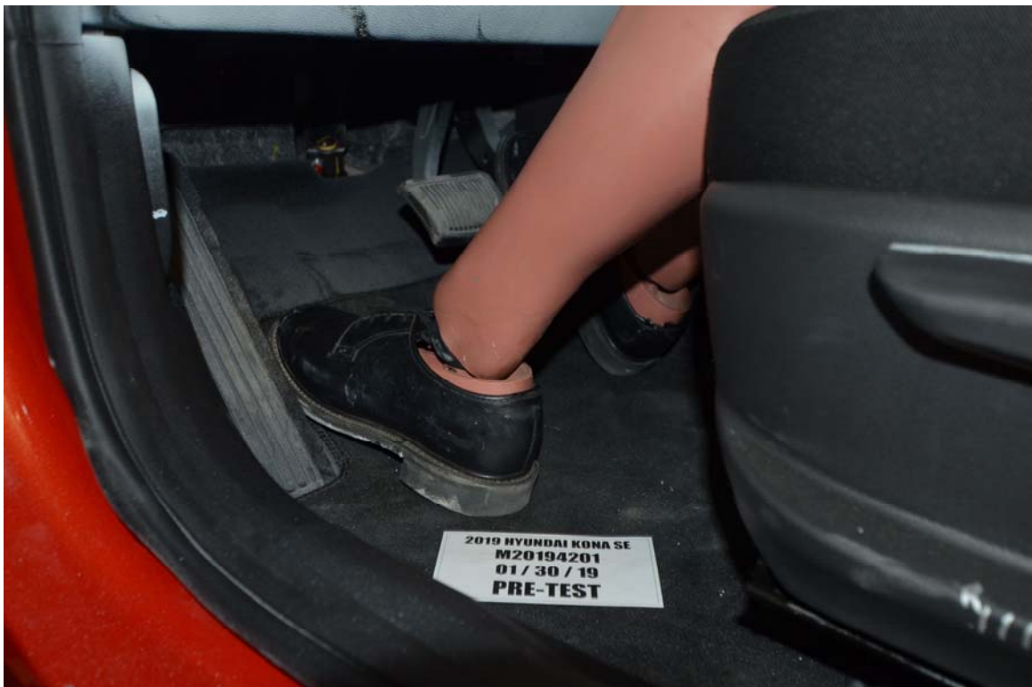
FIGURE 32. Pre-Test Placement of Dummy's Feet
