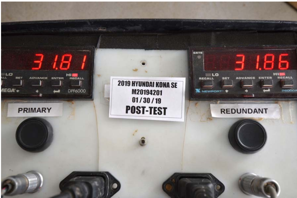
FIGURE 62. Post-Test Primary and Redundant Speed Trap Read-Out
