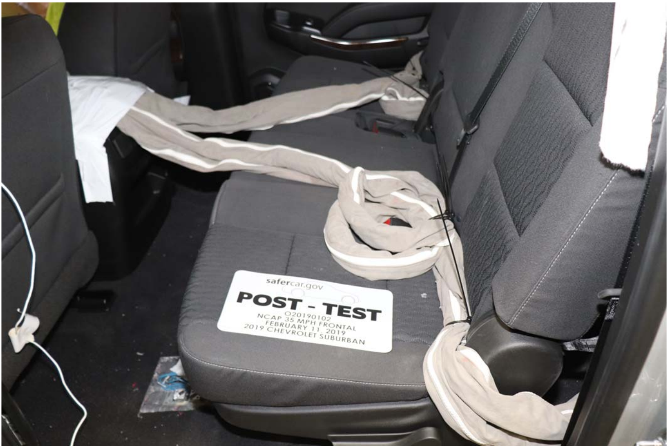
Photo No. 029 - Post-Test Dummy Cable Routing
