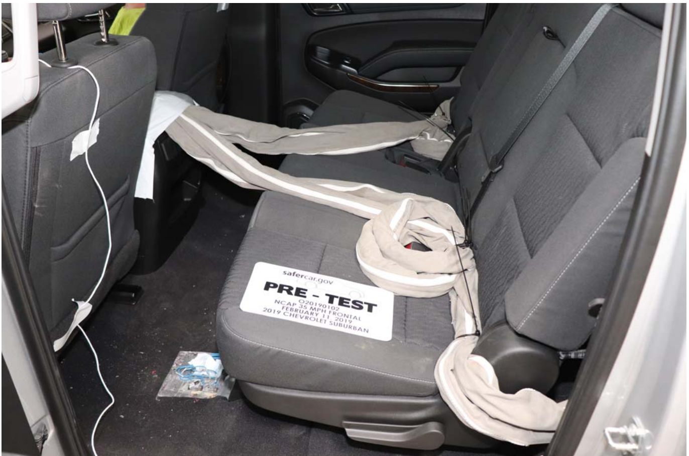
Photo No. 028 - Pre-Test Dummy Cable Routing
