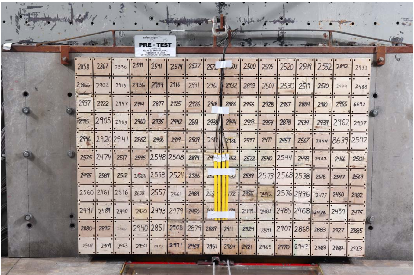
Photo No. 002 - Pre-Test Load Cell Wall
