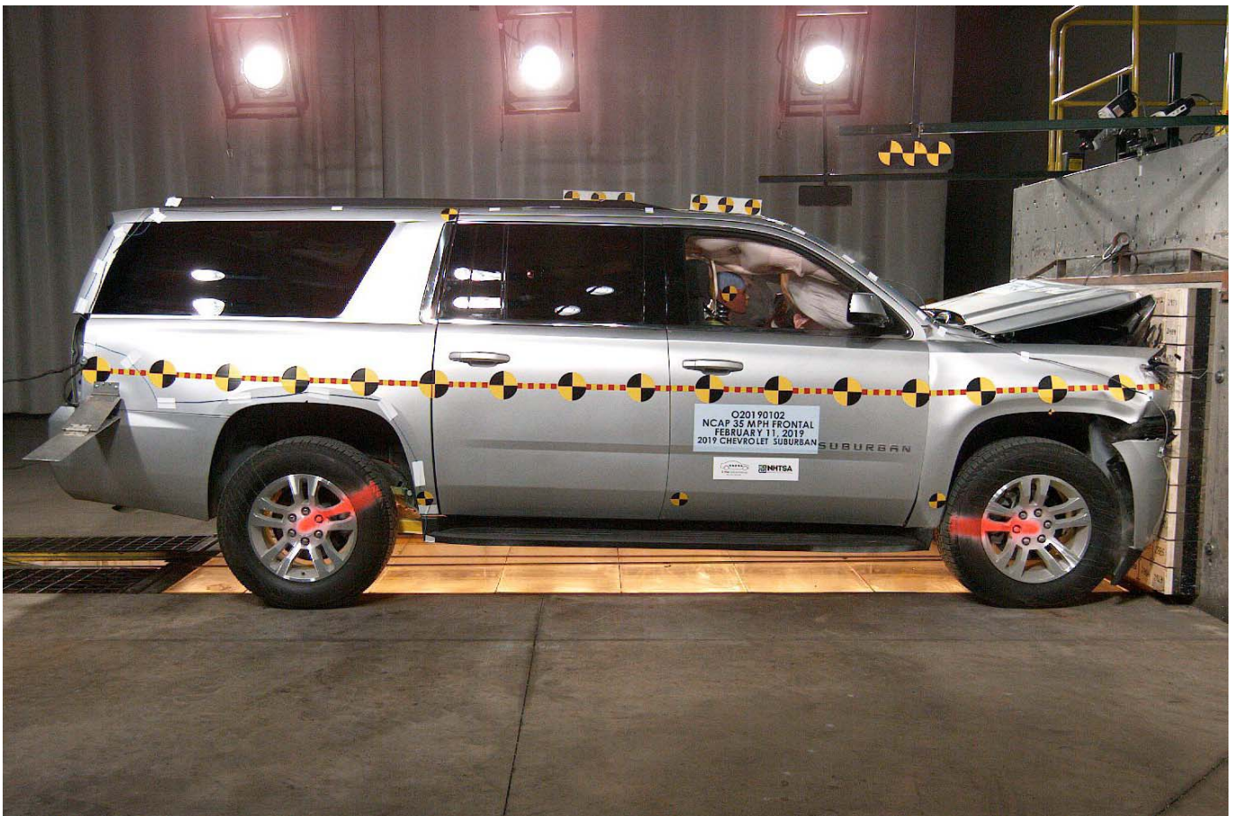
Photo No. 078 - 2019 Chevrolet Suburban 4WD LS 5-Door SUV Frontal Impact Event
