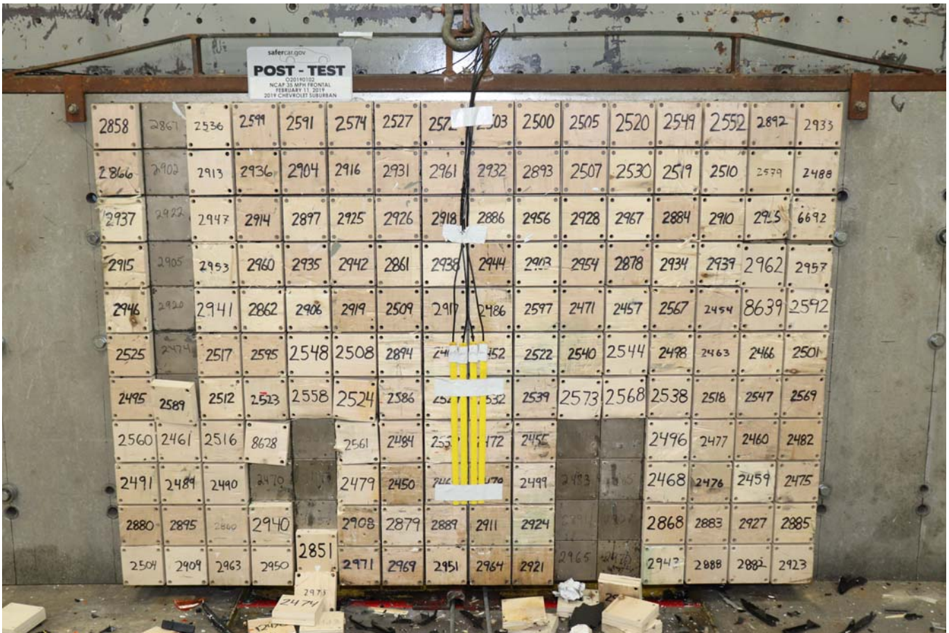
Photo No. 003 - Post-Test Load Cell Wall
