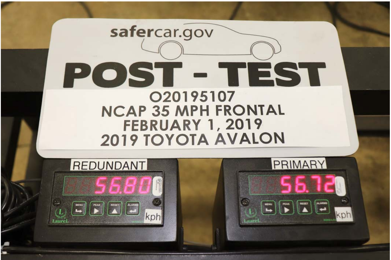
Photo No. 072 - Post-Test Speed Trap Read-Out
