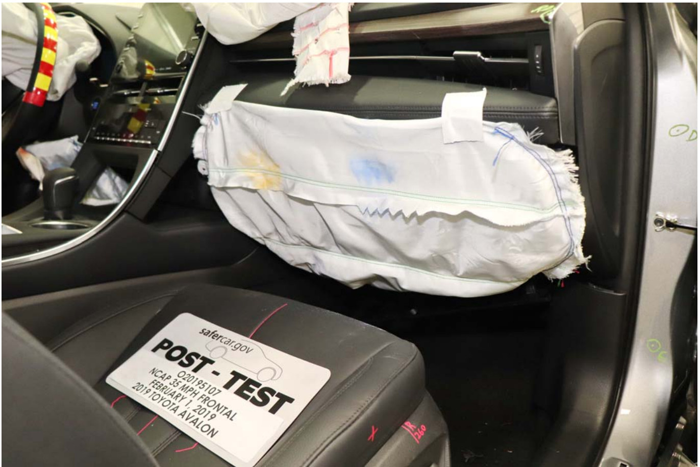
Photo No. 064 - Post-Test Passenger Side Knee Bolster
