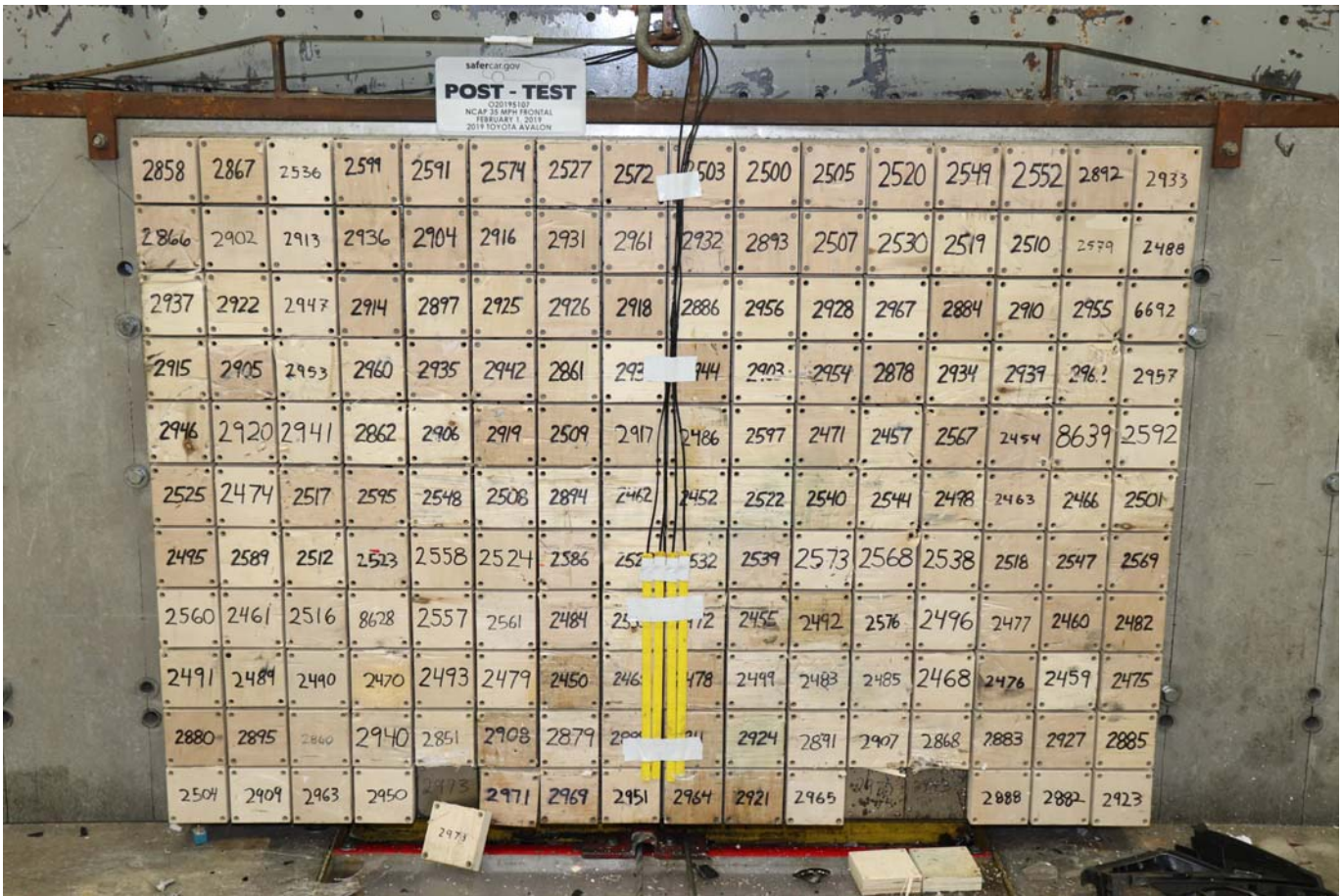
Photo No. 003 - Post-Test Load Cell Wall
