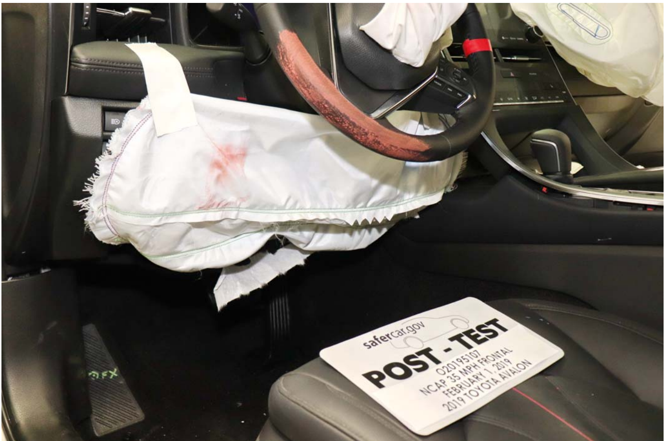
Photo No. 043 - Post-Test Driver Side Knee Bolster
