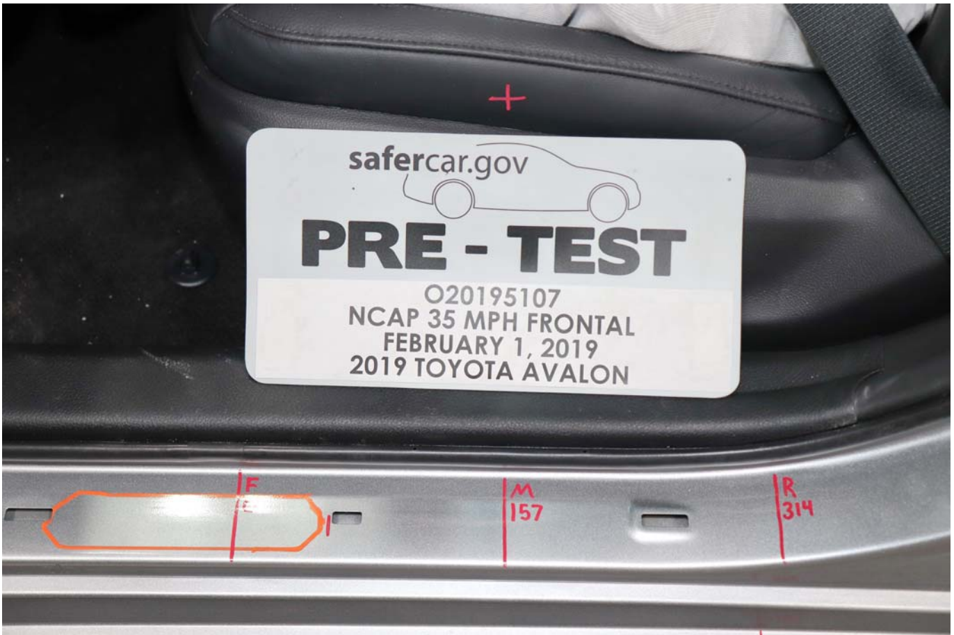
Photo No. 036 - Pre-Test Driver Seat Fore-Aft Markings
