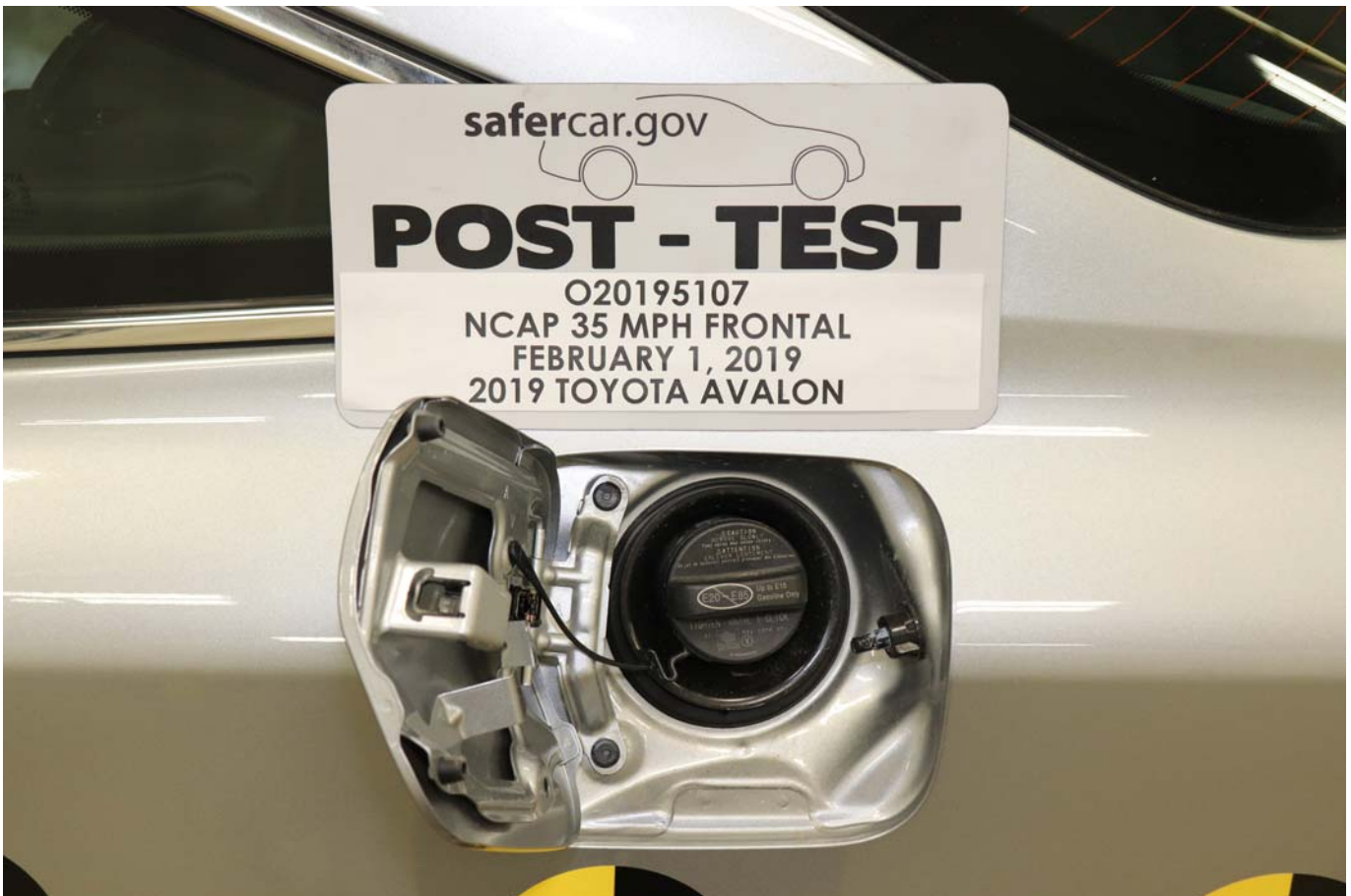
Photo No. 023 - Post-Test Fuel Filler Cap View
