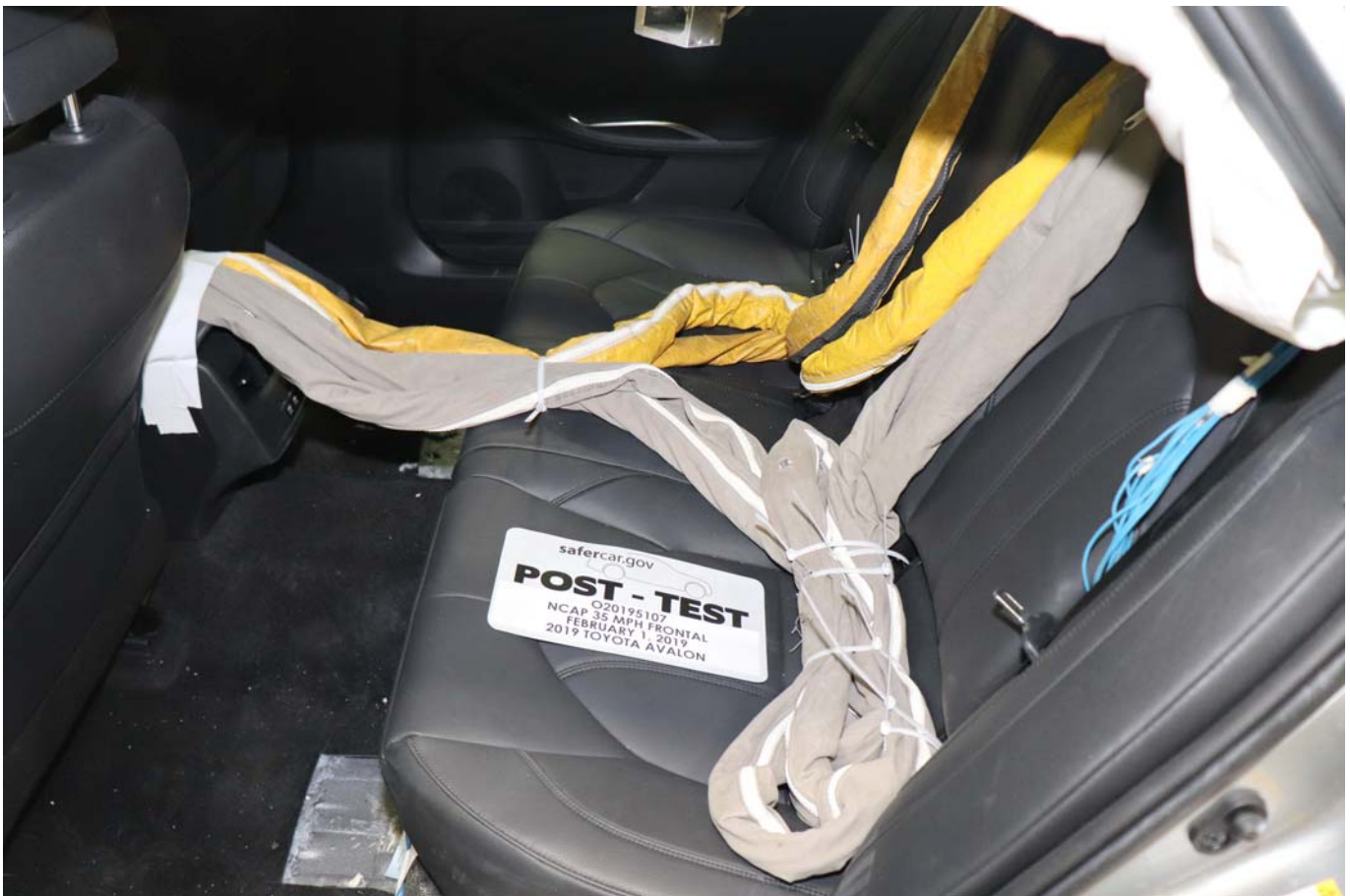
Photo No. 029 - Post-Test Dummy Cable Routing
