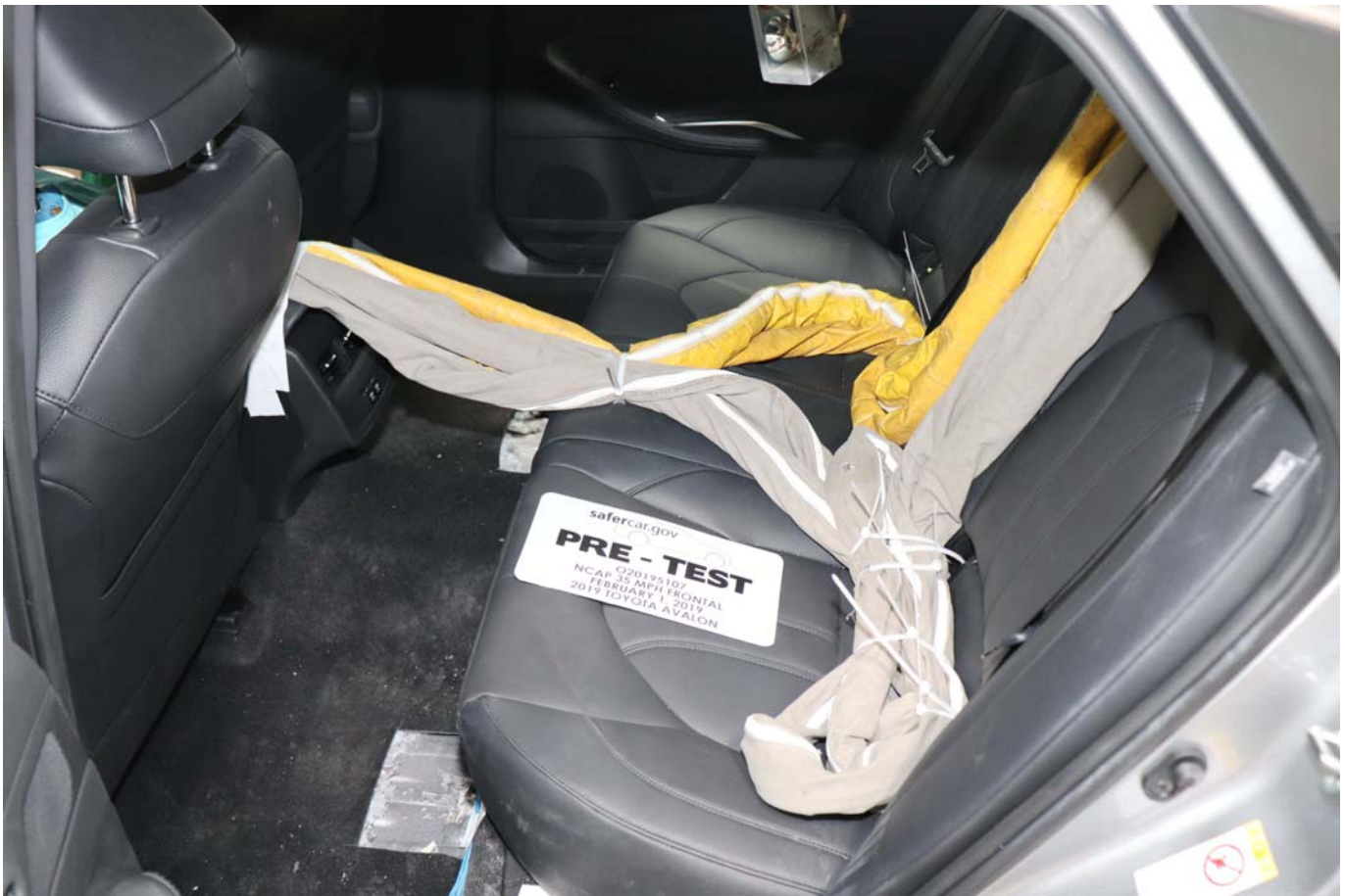
Photo No. 028 - Pre-Test Dummy Cable Routing
