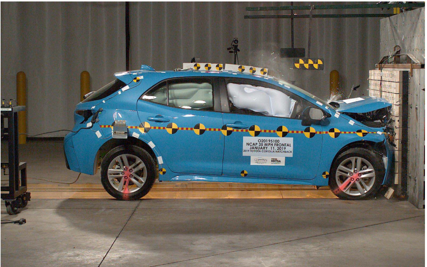
Photo No. 078 - 2019 Toyota Corolla Hatchback SE 5-Door Hatchback Frontal Impact Event
