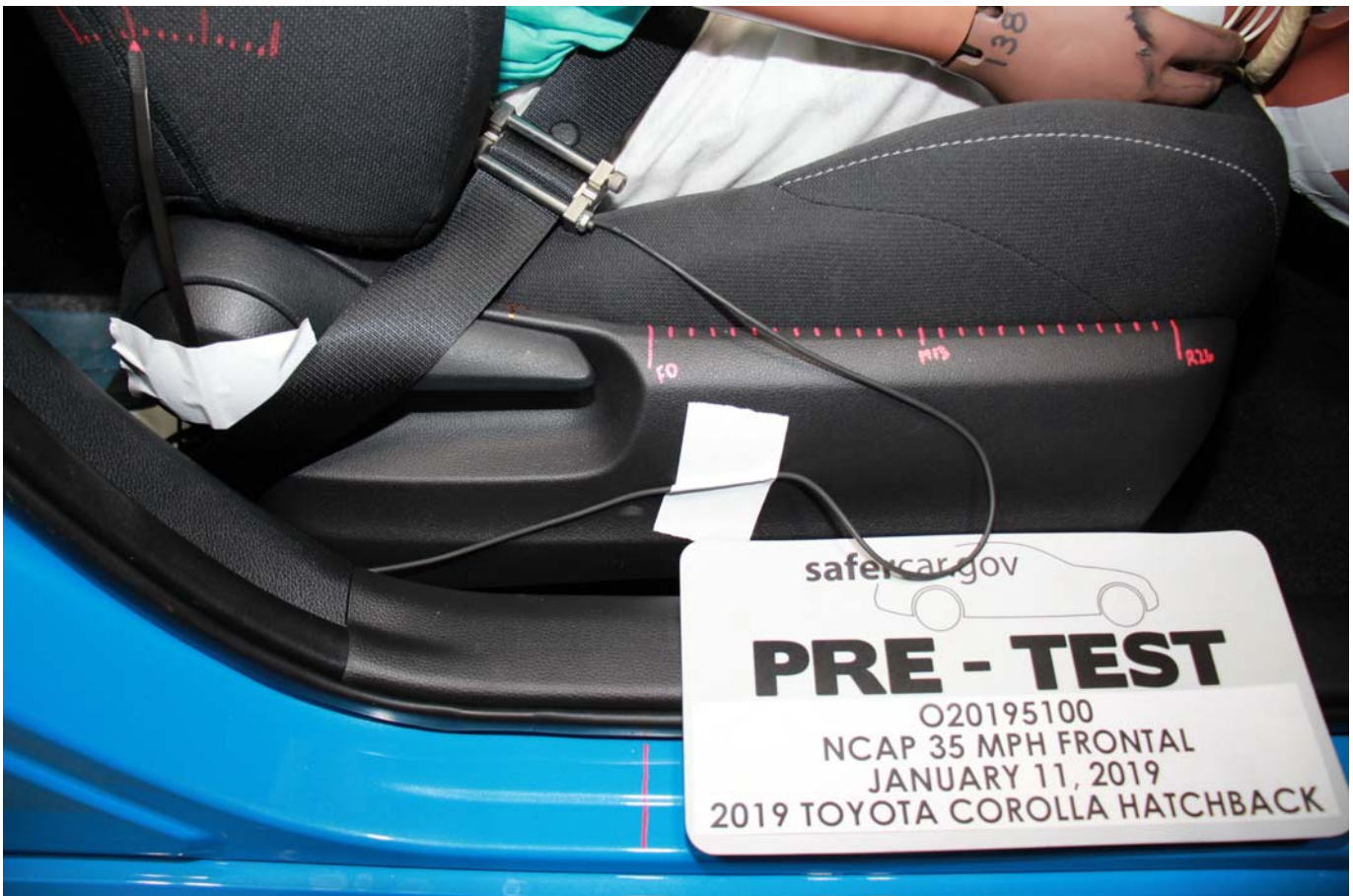
Photo No. 057 - Pre-Test Passenger Seat Fore-Aft Markings
