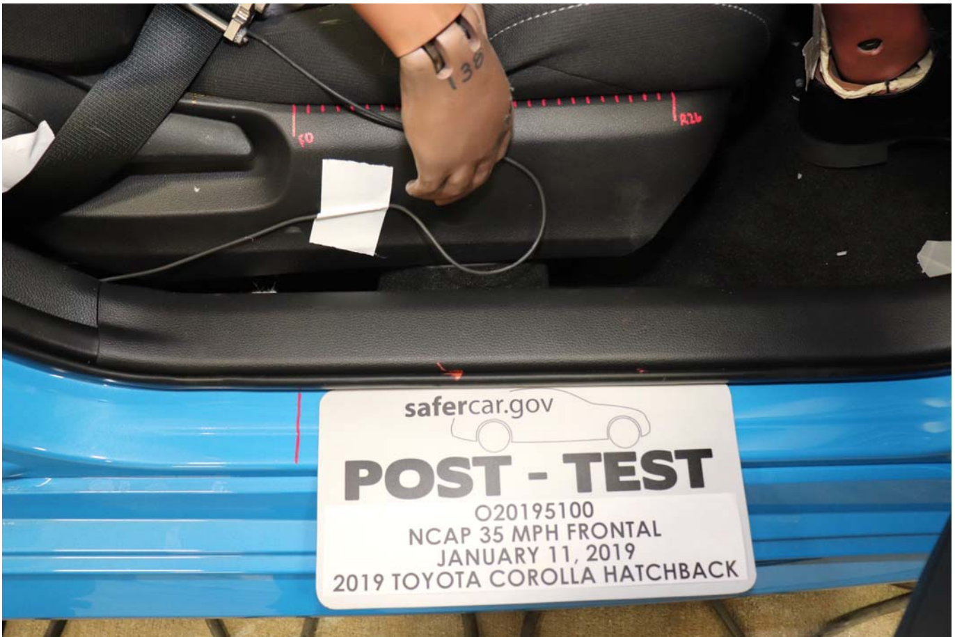
Photo No. 058 - Post-Test Passenger Seat Fore-Aft Markings
