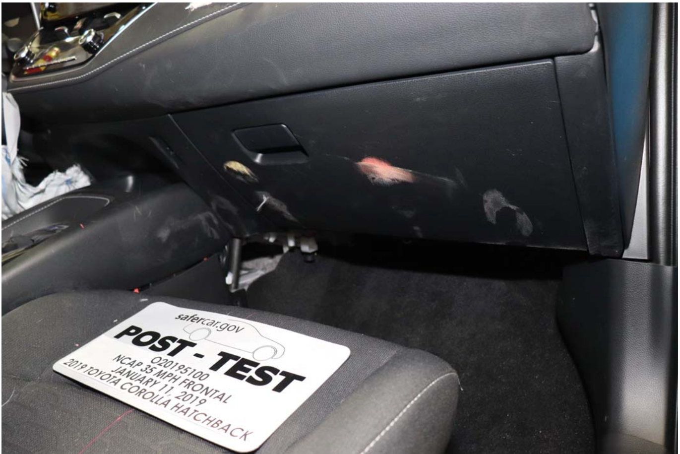
Photo No. 064 - Post-Test Passenger Side Knee Bolster
