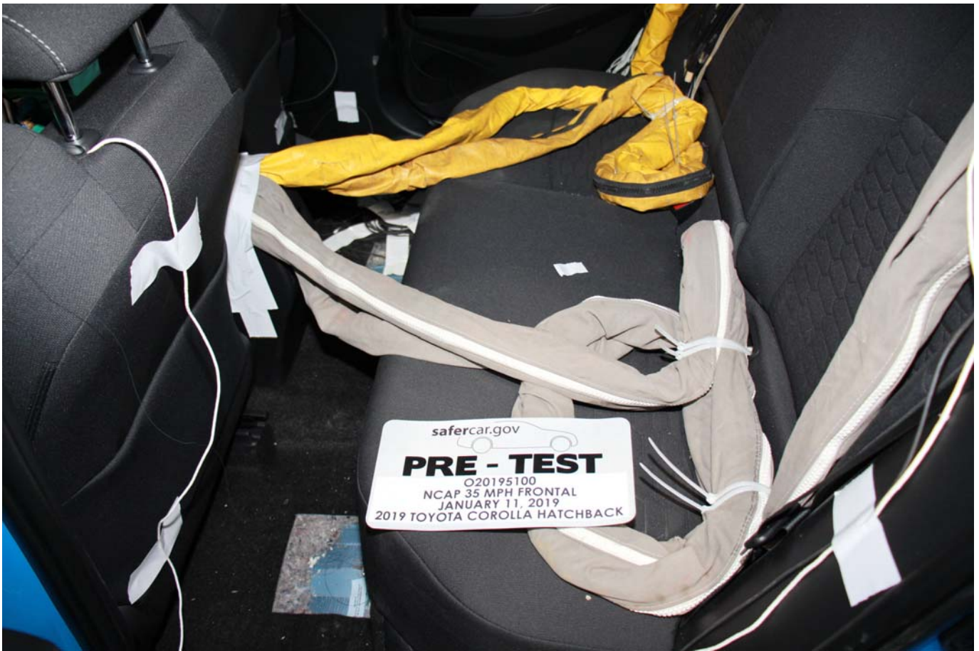
Photo No. 028 - Pre-Test Dummy Cable Routing
