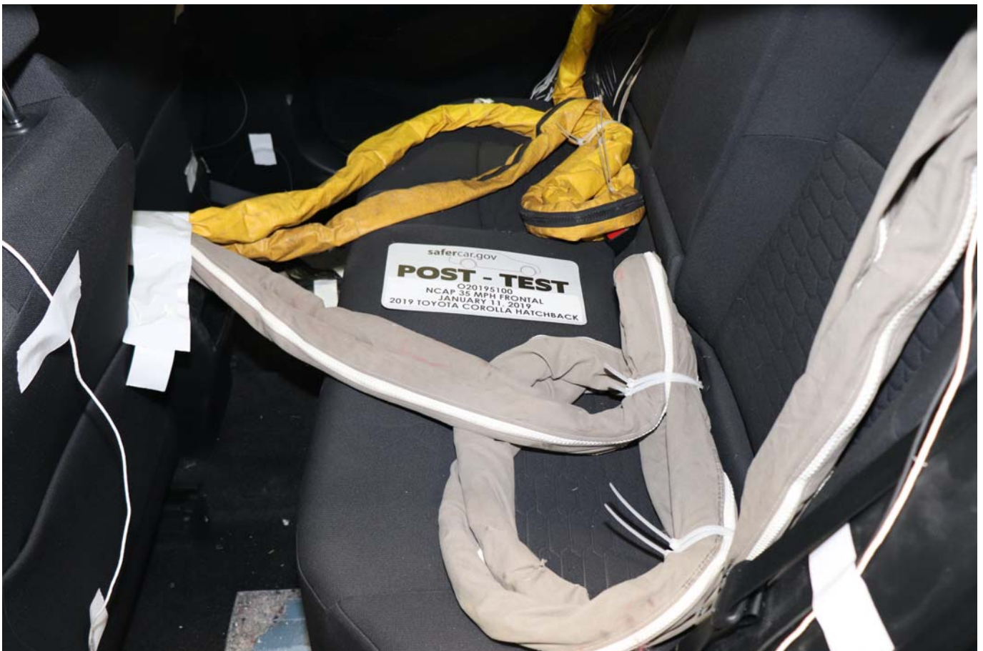
Photo No. 029 - Post-Test Dummy Cable Routing
