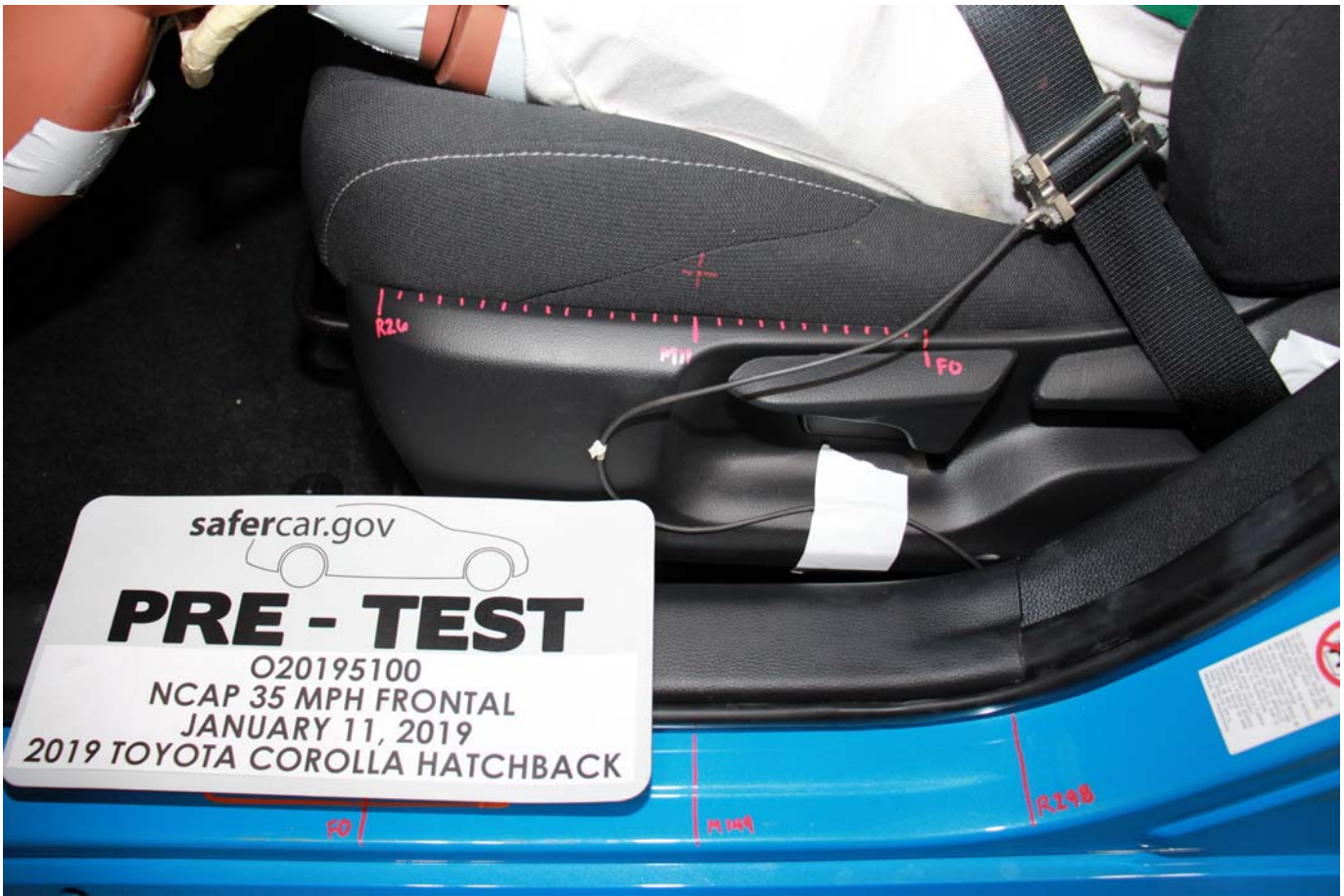
Photo No. 036 - Pre-Test Driver Seat Fore-Aft Markings
