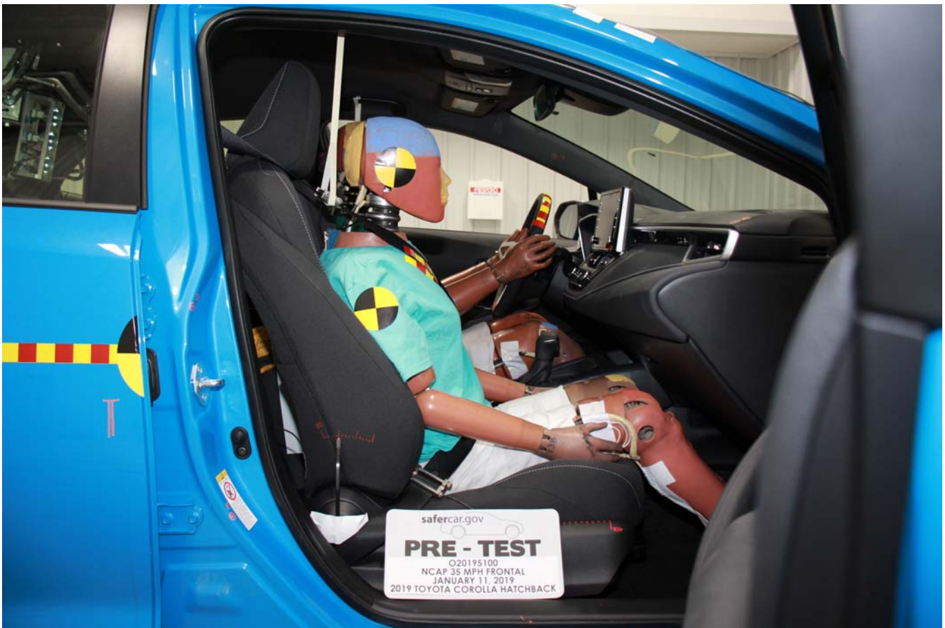
Photo No. 055 - Pre-Test Passenger Dummy and Vehicle Interior
