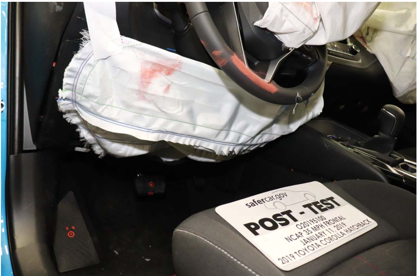
Photo No. 043 - Post-Test Driver Side Knee Bolster
