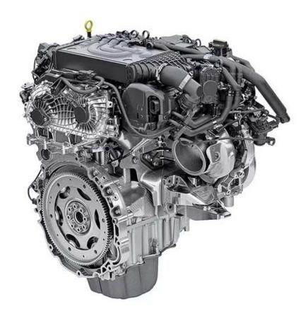
Jaguar Land Rover's 3.0-liter Ingenium six-cylinder engine, below, is to debut this spring in the 2019 Range Rover Sport.
