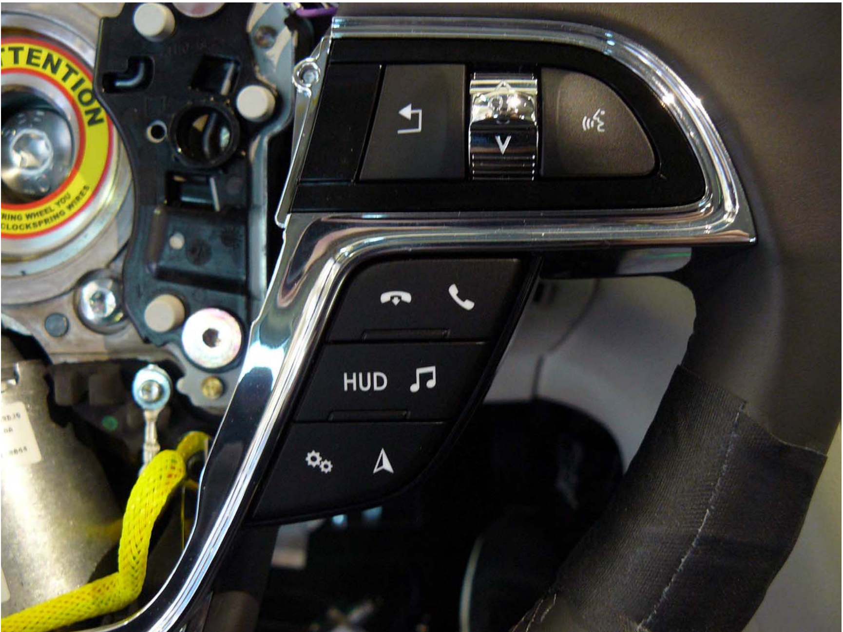
Figure A18. Steering Wheel Mounted Controls for Changing Parameters
