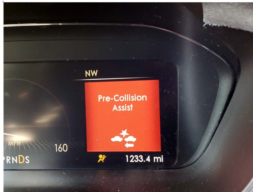
Figure A16. Instrument Panel AEB Visual Alert
