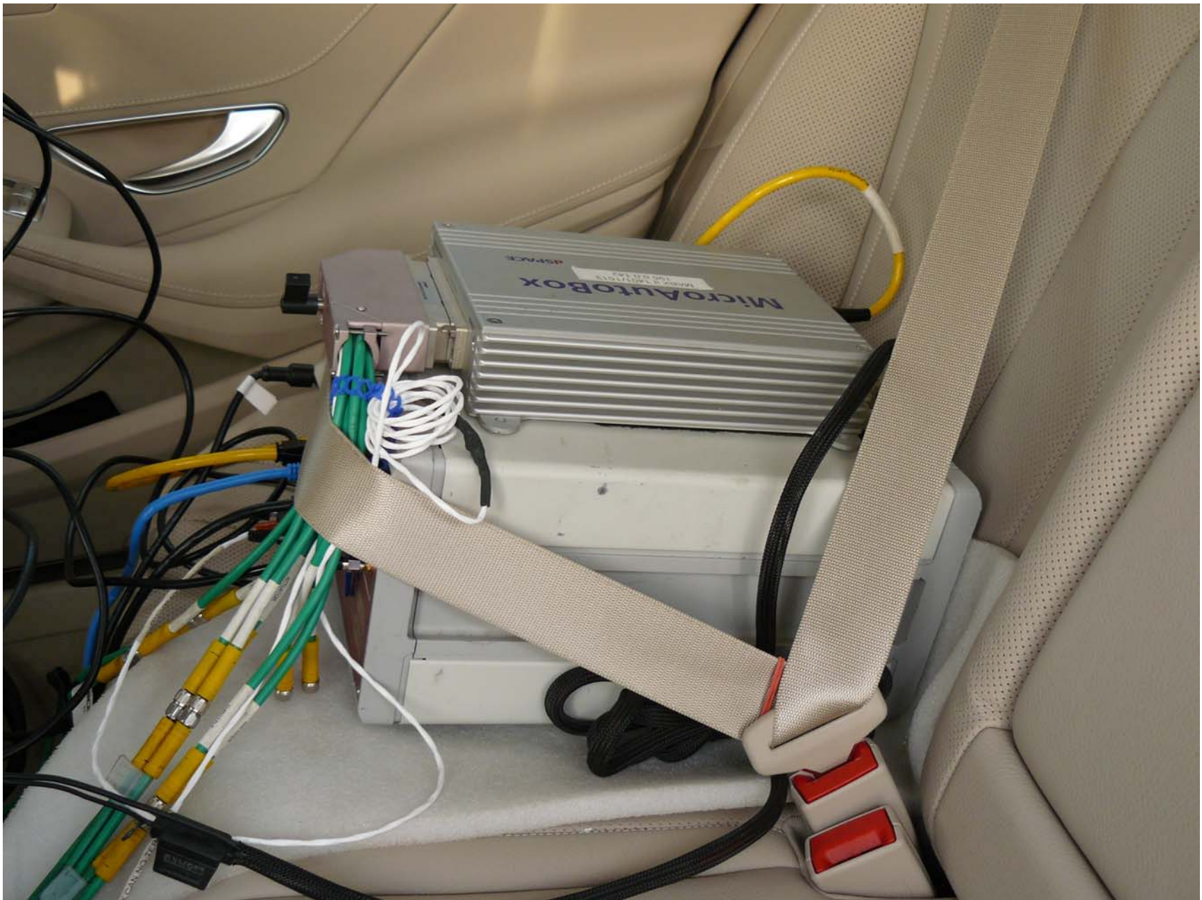
Figure A11. MicroAutoBox Installed in Subject Vehicle
